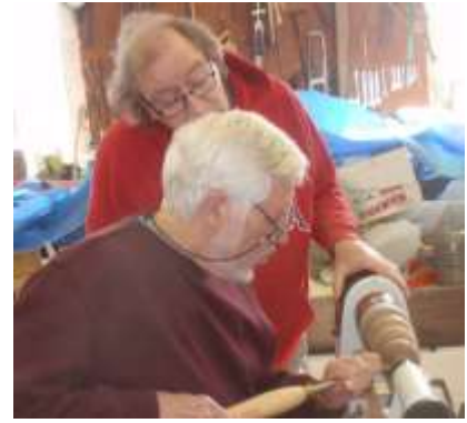
Len has Fred Johnson's attention with his technique on cutting coves on the lathe.
