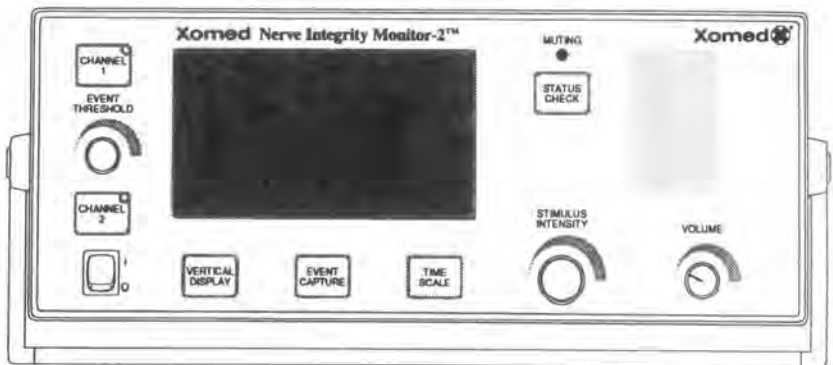
FIGURE 3-1. The Nerve Integrity Monitor-2 (NIM-2, Xomed-Treace, Inc., Jacksonville, Florida) directs detected EMG activity to an oscilloscope that generates a visual representation of muscle activity on a central screen.
