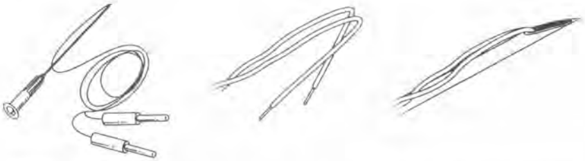
FIGURE 4-3. Bipolar hook wire electrodes for recording EMG potentials. From "Facial Nerve Electrophysiology: Electroneurography and Facial Nerve Monitoring" by D. L. Beck, 1993, Seminars in Hearing , 14, p. 129. Copyright 1993 by Thieme Medical Publishers. Reprinted with permission.
