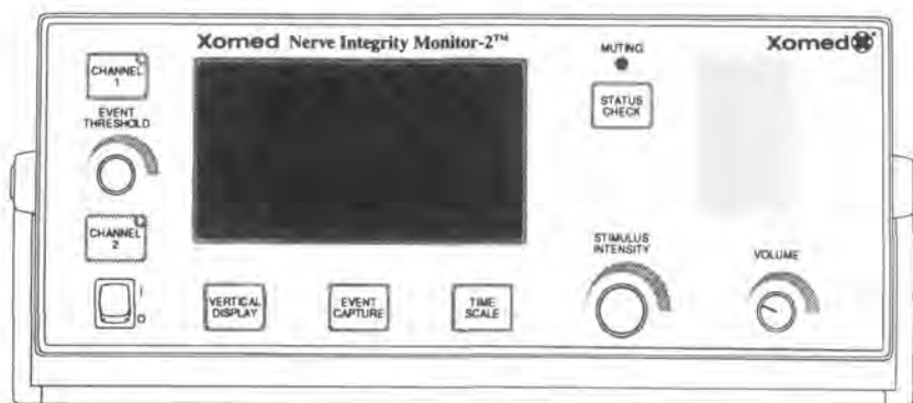
FIGURE 2-1. Front panel of the Nerve Integrity Monitor-2 (NIM-2, Xomed-Treace, Inc., Jacksonville, Florida). Touch pads on the right side of the device allow for simultaneous monitoring of up to two channels.
