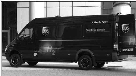
UPS will use this fuel cell-powered Dodge Sprinter in delivery service in Los Angeles.
