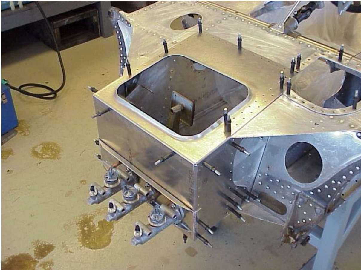
This photo shows the work required to let in extra panels to the front footbox of 56/1 during restoration to accommodate Bruce Linsmeyer's height.
