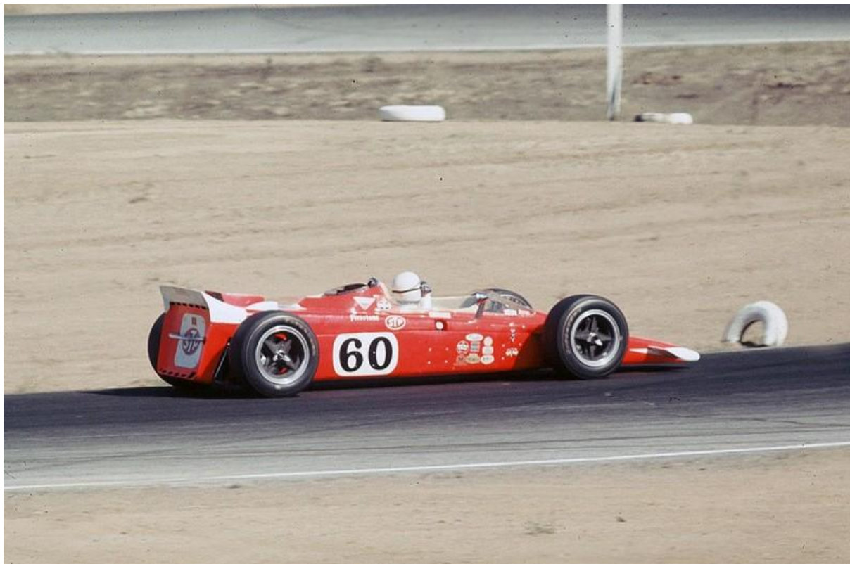
Leonard at Riverside, December 1 st 1968, 56/1's last appearance in turbine form. Note distinctive cooling slots in the rear panel (seven in the top – of which six are visible in this shot – and four in the bottom plus a fifth larger, square hole bottom right). Right-hand side fuel filler is also visible.
