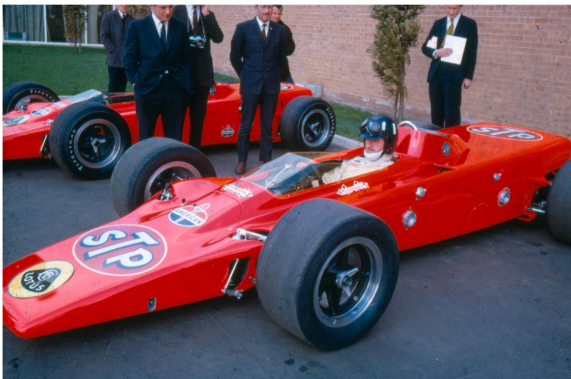
This I believe, shows Graham Hill at the April 1968 press launch in 56/1, with 56/2, returned from testing at Indy, and with a new Naca duct at the rear to feed air to the rear brakes, alongside.
