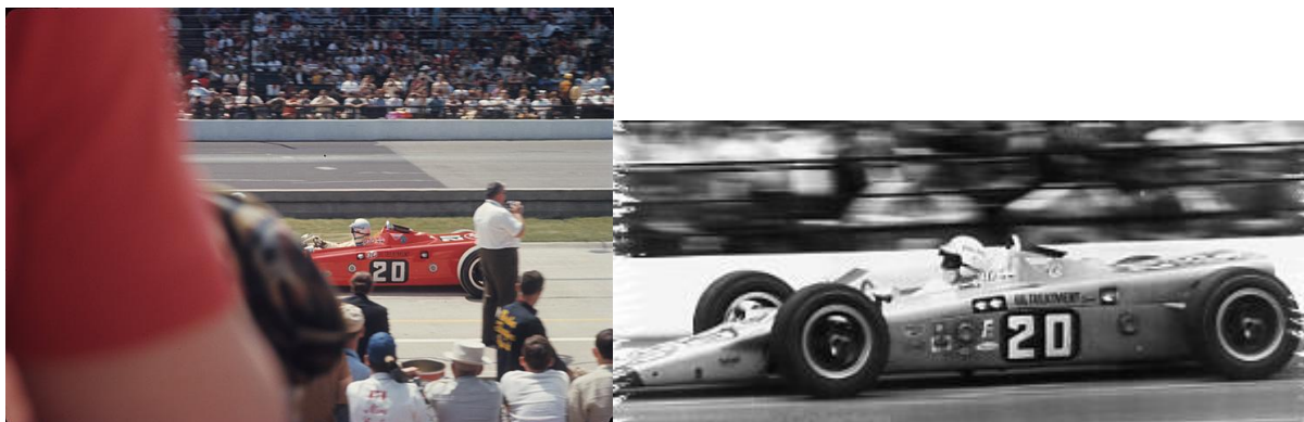
A comparison of 56/4 on qualification day (left) with the single fuel filler (just level with the driver's helmet) and in the race (right) with the double fuel filler arrangement.
