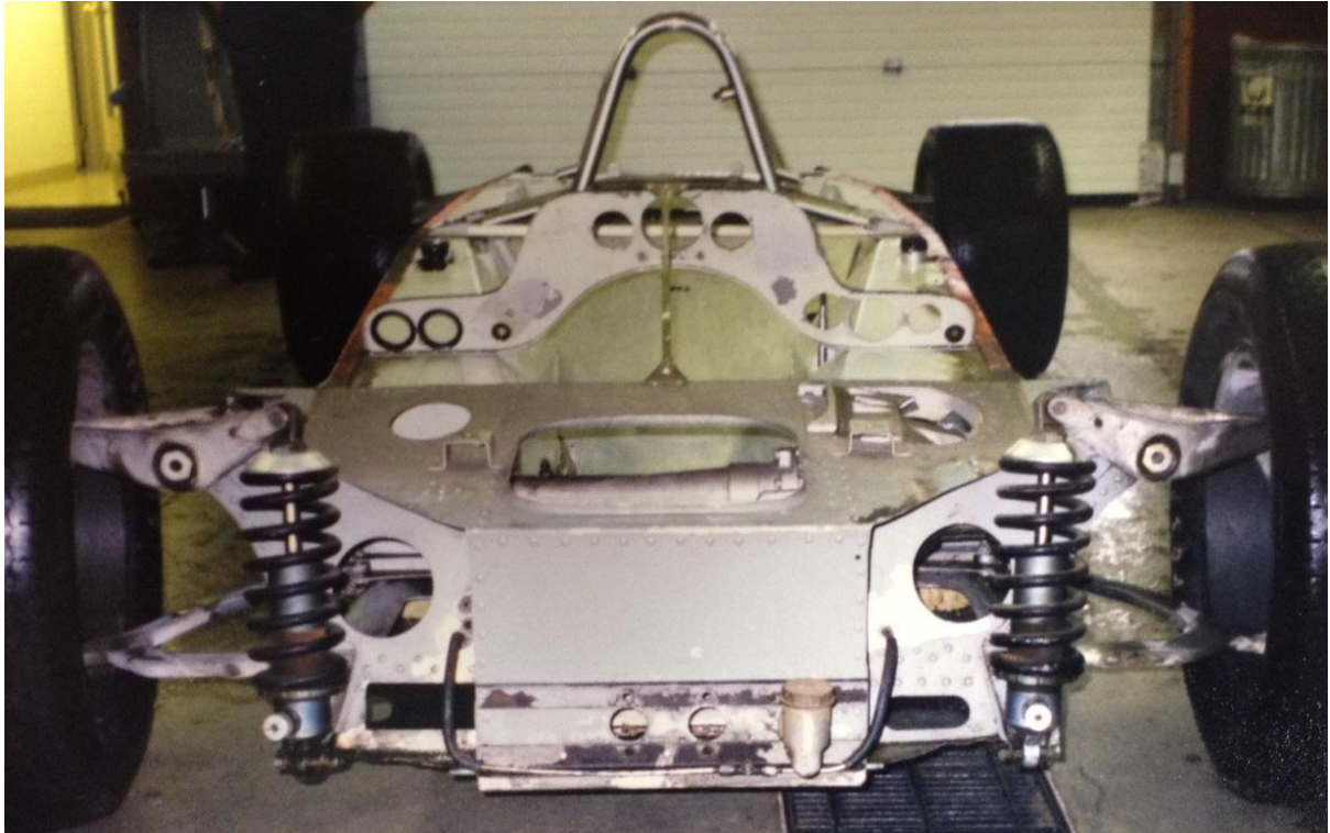
This photo shows the front footbox area of the car when it was received by Linsmeyer, although it is considerably different to photos of 56/1 taken at the 1968 Indy 500 (see below). Visible are the triangular fitments for the dash fixtures – three rivets where it fits to the dash plate and two where it fits to the footbox.
