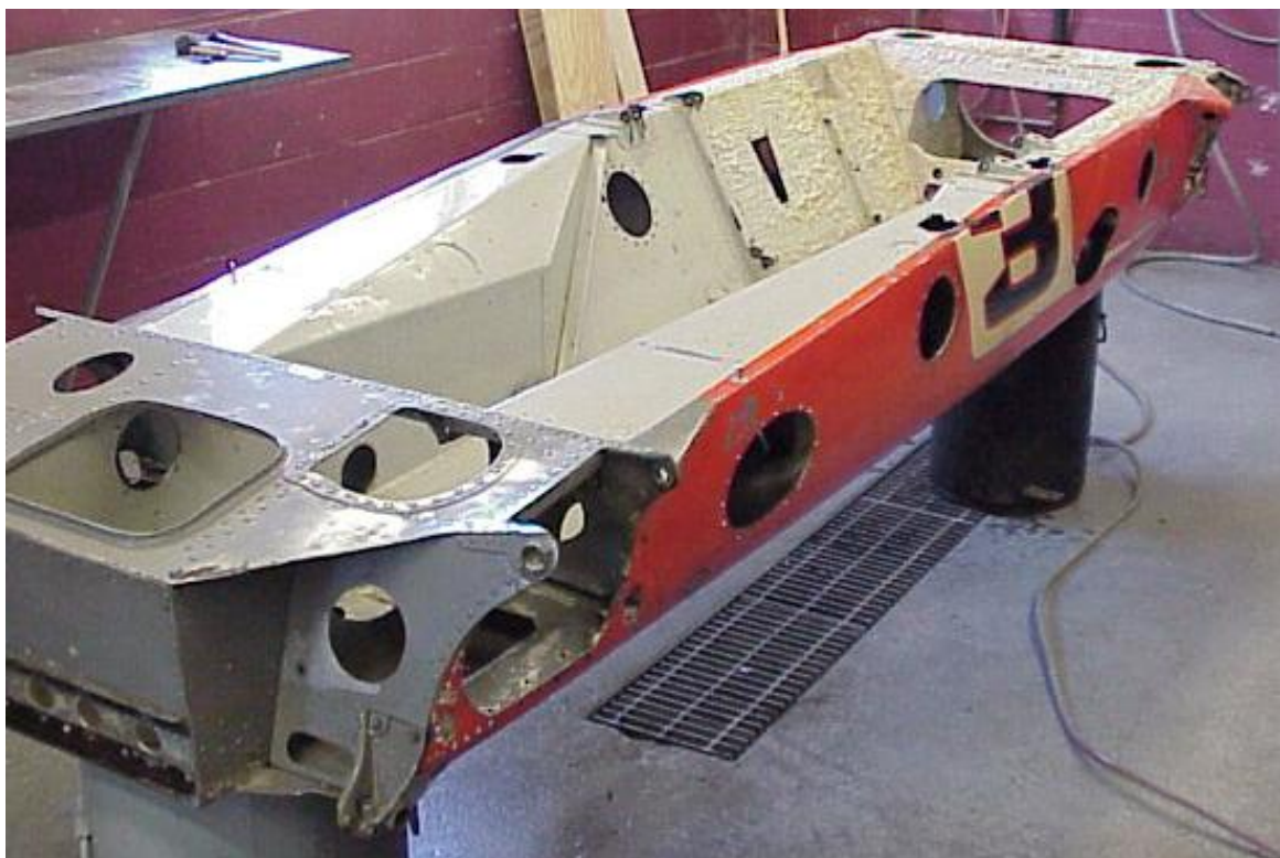
Holes for dry-break fuel couplings and fuel tank access hatches are in the correct location for the Lotus 56.
