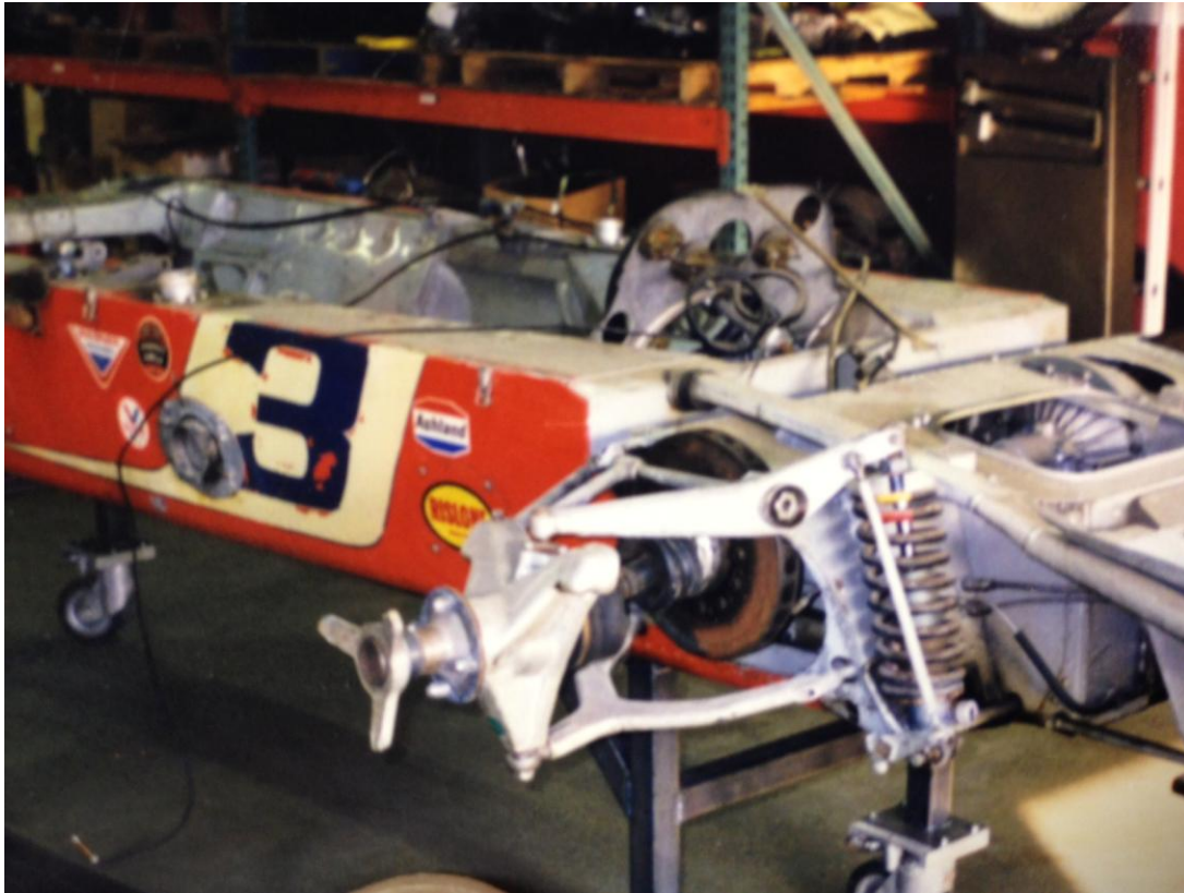
The VPJ copy (which ran the normally aspirated four-cam Ford engine) was a crude attempt to mimic a Lotus 56 chassis, with flat sides and a dash plate sunk in to the cockpit sides, rather than sitting atop them. It is shown here after Linsmeyer had bought it and before he swapped cars with Winslow.
