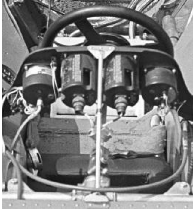
Lotus-built 56s feature triangular plates at both ends of the brace between the dash plate and the footbox. This shot shows 56/1 but all works cars had the same fitting.
