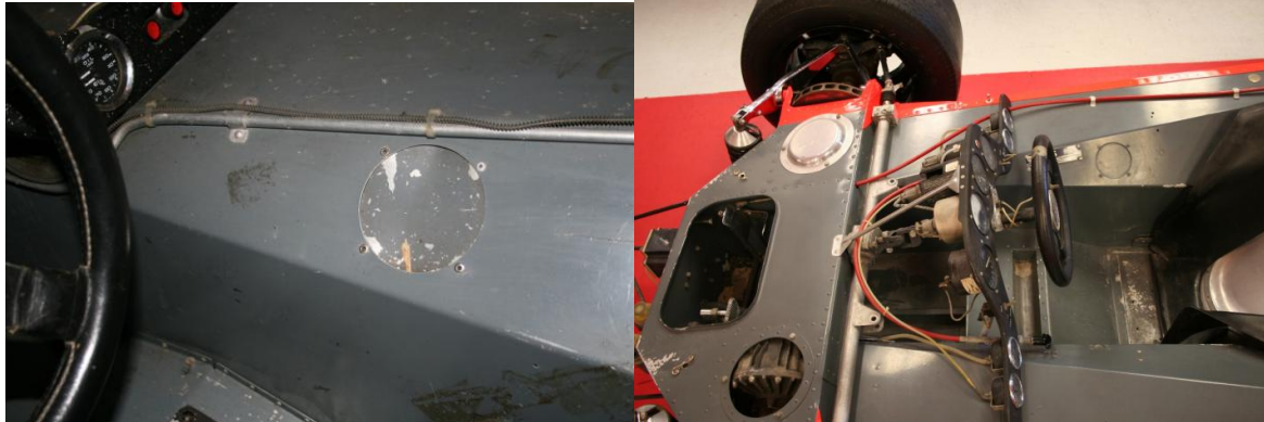
The blanked-off gauge hole in the tub of the 56B/1 Formula 1 turbine car (left). Interestingly, the absence of holes for a chassis plate (which was mounted on the opposite cockpit panel on this car) could suggest that it was not originally one of the original four '68 Indy cars but a newly-built chassis. 56/3 (right) still features the blanked-off hole today.
