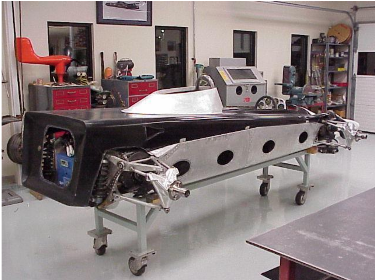
This photo, taken during the restoration process, shows the right-hand side skins of the car with the correct four fuel tank access hatches.
