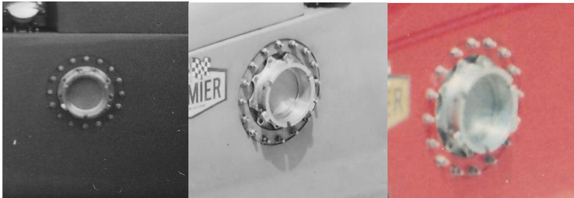
Several different views of the Avery-Hardoll dry-break fuel couplings used on the Lotus 56. They were all secured by 16-bolt fixings.
