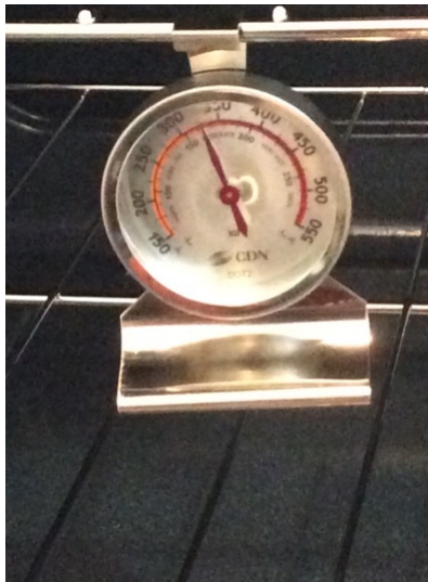
Tested oven, cooked at 330° when set at 350°
