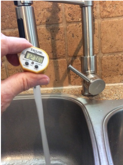
Hot water temperature 127°
