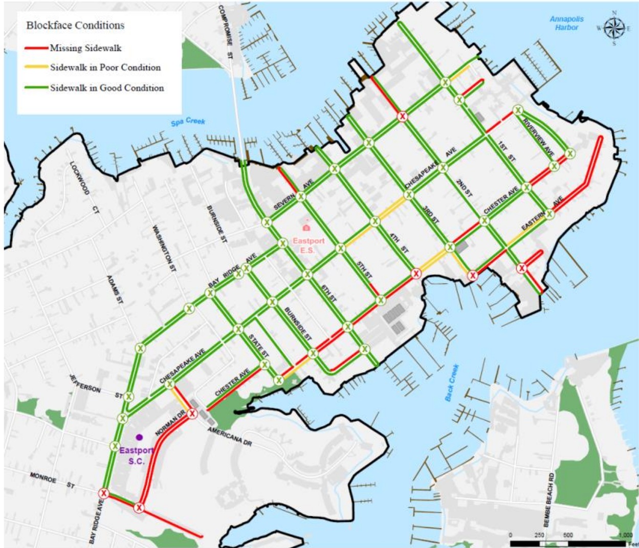
Figure 16: Locations where is sidewalk is in poor condition or missing
