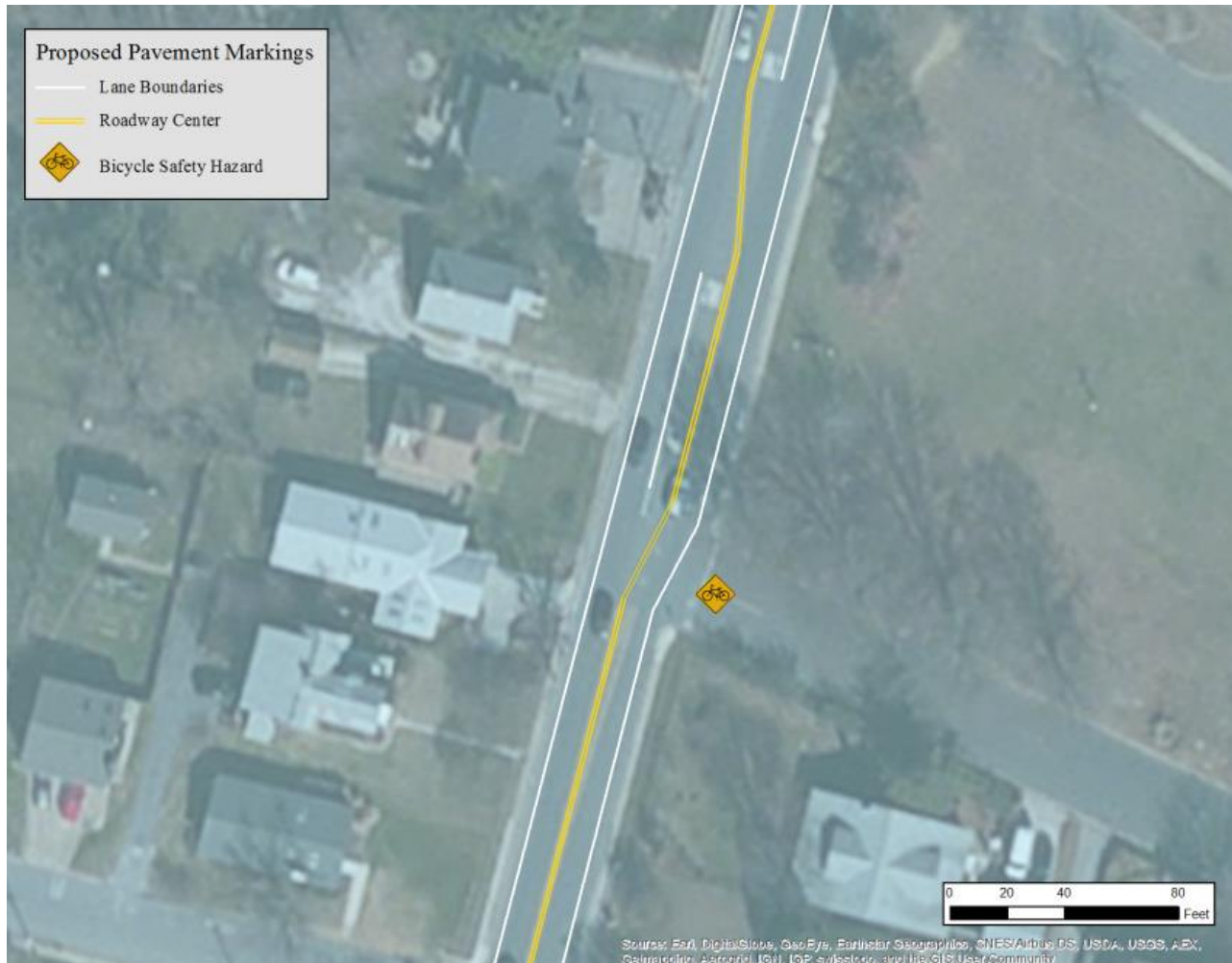
Figure 11: Gradual transition of lane shifts along Bay Ridge Avenue between Fairview and Springfield
