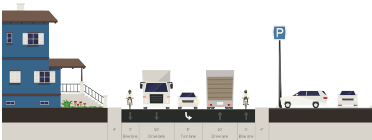
Figure 10: Existing and proposed lane use along Bay Ridge from Chesapeake to Fairview
