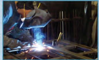
All mitred corners and each steel joint is welded at over 1000 degrees to form a solid piece of steel for structural integrity.
