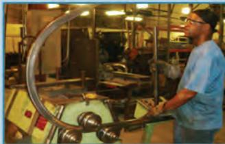
The steel is then skillfully punched, drilled, rolled and twisted to create intricate and unique designs.
