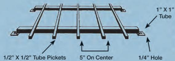
Home Guard steel window guards are constructed using 1/2" square steel tube pickets welded to 1" square steel tube crossbars providing both exceptional strength and security. Pickets are spaced approximately 5" on center. All window guards exceeding 48" in height will have an additional 1" crossbar added to them to provide greater strength and stability to the window guard. All window guards are powder coated to provide a durable and beautiful finish.
