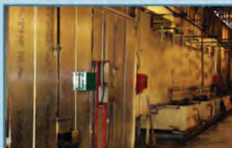
Each door then enters a five stage wash system where they are degreased, rinsed, phosphated and sealed prior to powder coating.
