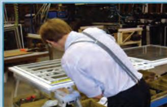
In final assembly the doors are outfitted with custom hardware, glass, screens and frames, then closely inspected for quality assurance.
