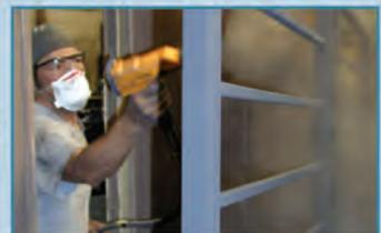
Every door is then grounded to create a magnetic charge to attract and hold the polyester powder coating until it reaches the oven.
