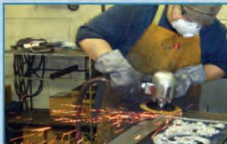
After welding, grinders hand smooth each weld with three different types of abrasives until the joints are silvery smooth.
