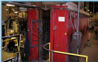
In the oven all doors are heated to 425 degrees for a period of twenty minutes to fuse the powder with the metal surface.
