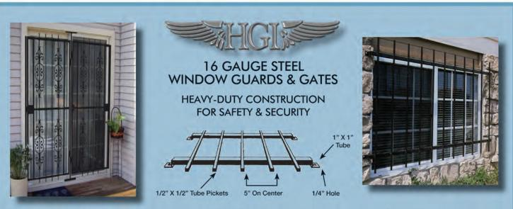
Home Guard steel window guards are constructed using 1/2" square steel tube pickets welded to 1" square steel tube crossbars providing both exceptional strength and security. Pickets are spaced approximately 5" on center. All window guards exceeding 48" in height will have an additional 1" crossbar added to them to provide greater strength and stability to the window guard. All window guards are powder coated to provide a durable and beautiful finish.
