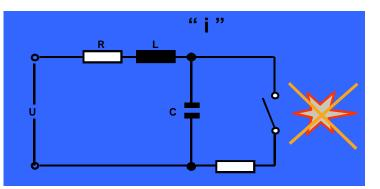
The energy in an intrinsically safe system is limited to a value that is not capable of causing ignition in normal operation and fault condition in the surrounding hazardous atmospheres by sparks (opening, closing, short circuit, short circuit to earth)
