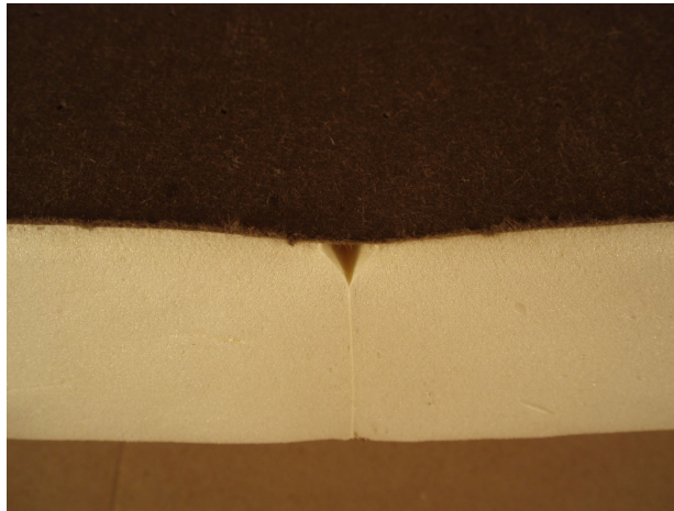
Knit line and V-groove close-up (after conditioning)
