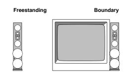
Boundary placement refers to a situation in which the XA Tower is bounded on at least one side by a large object.
