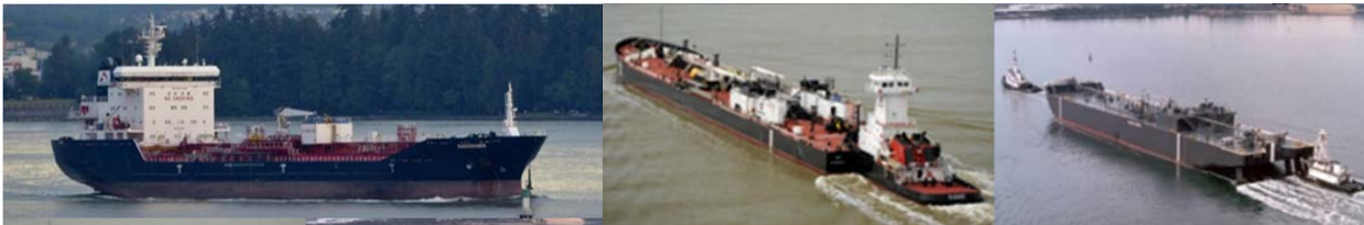
Vessels identified in ESHB 1578. Left: a 17,000 DWT oil tanker (photo M.L. Jacobs), a Crowley ATB (photo Crowley.com), Right: a towed oil barge (photo Sause.com)
