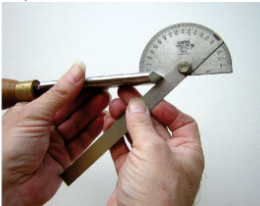
Fig 2 – Measuring edge angle
