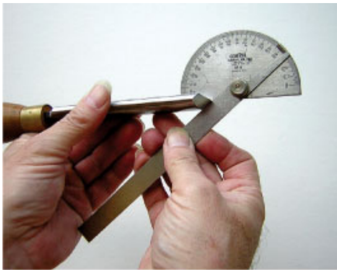
Fig 2 – Measuring edge angle
