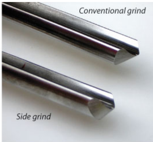
Fig 7 – Side grind produces a conical bevel
