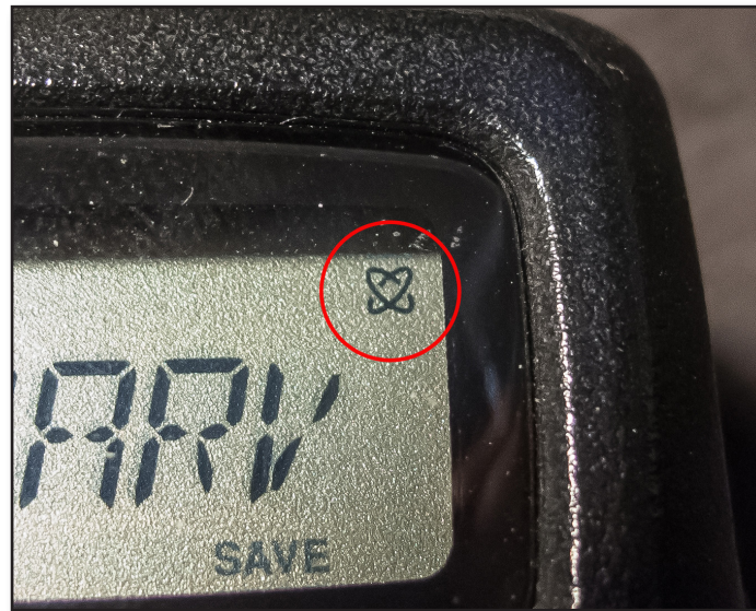
The WIRES Symbol as it appears on the screen of a Yaesu FT-60 handheld. This may appear differently on differet radios. Refer to the manual to be sure.
