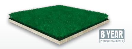
**DROPTURF** features a 40 oz. textured polyethylene that offers excellent ball roll. DropTurf provides a much less abrasive surface than nylon or polypropylene and provides superior wear resistance. DropTurf is 19 mm thick, combining the 14 mm polyethylene turf with a 5 mm foam backing, providing superior safety and performance. Thicker backing options are available via custom order.
