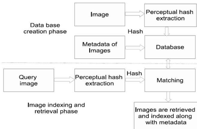
Figure 5.3: Block diagram of perceptual hashing based image indexing and retrieval application.
