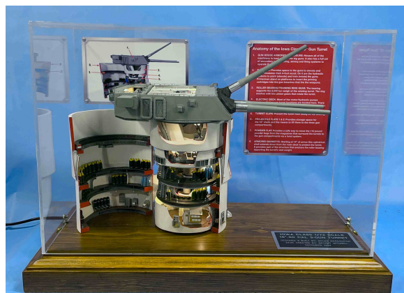
IMAGE 2: "1:48 Scale Model of Entire 5"/38Cal Secondary Battery System."
