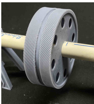
Image 15: "Successful Assembled Bull Gear Test Fit on PCVC 5/8" Pipe Serving as the Propeller Shafts."
