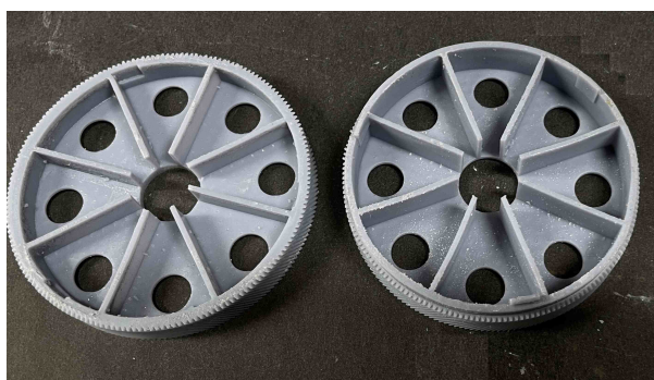
Image 16: "Bull Gear Print Showing Both Halves and Internal Ribbing That Prevented Warping."
