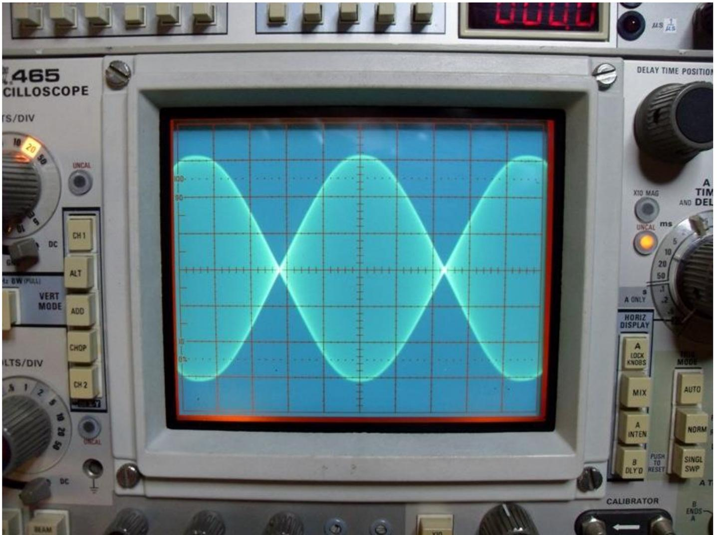
**Figure 14: Two Tone Scope Pattern at RF Output**
