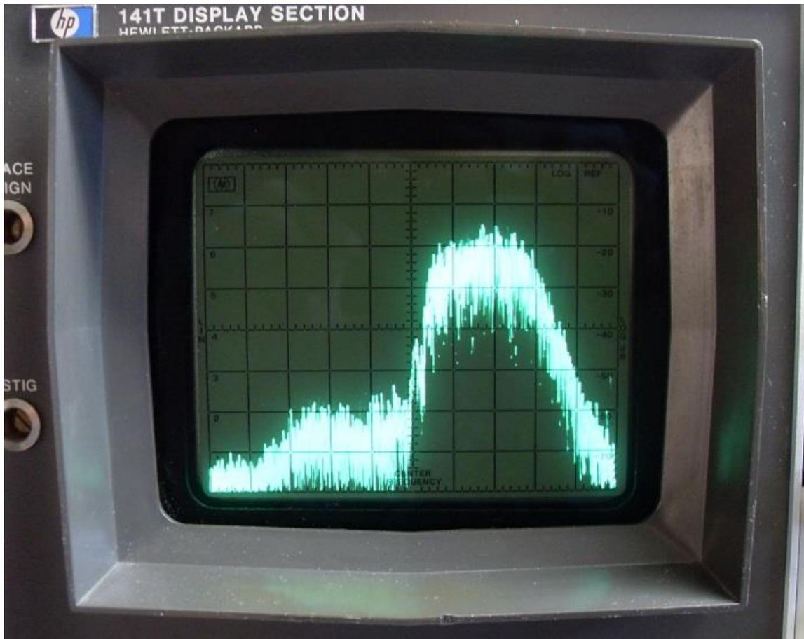
**Figure16: This was done just for fun to see what would happen. I tuned an FM radio off station so it would produce white noise and put the transmitter's mic against the speaker. Then I looked at the RF spectrum at the dummy load on my old HP spectrum analyzer. The carrier is at the center and each horizontal division is 1 kHz. You can clearly see the audio (and resultant RF) passband is about 2.5 kHz wide just as predicted.**
