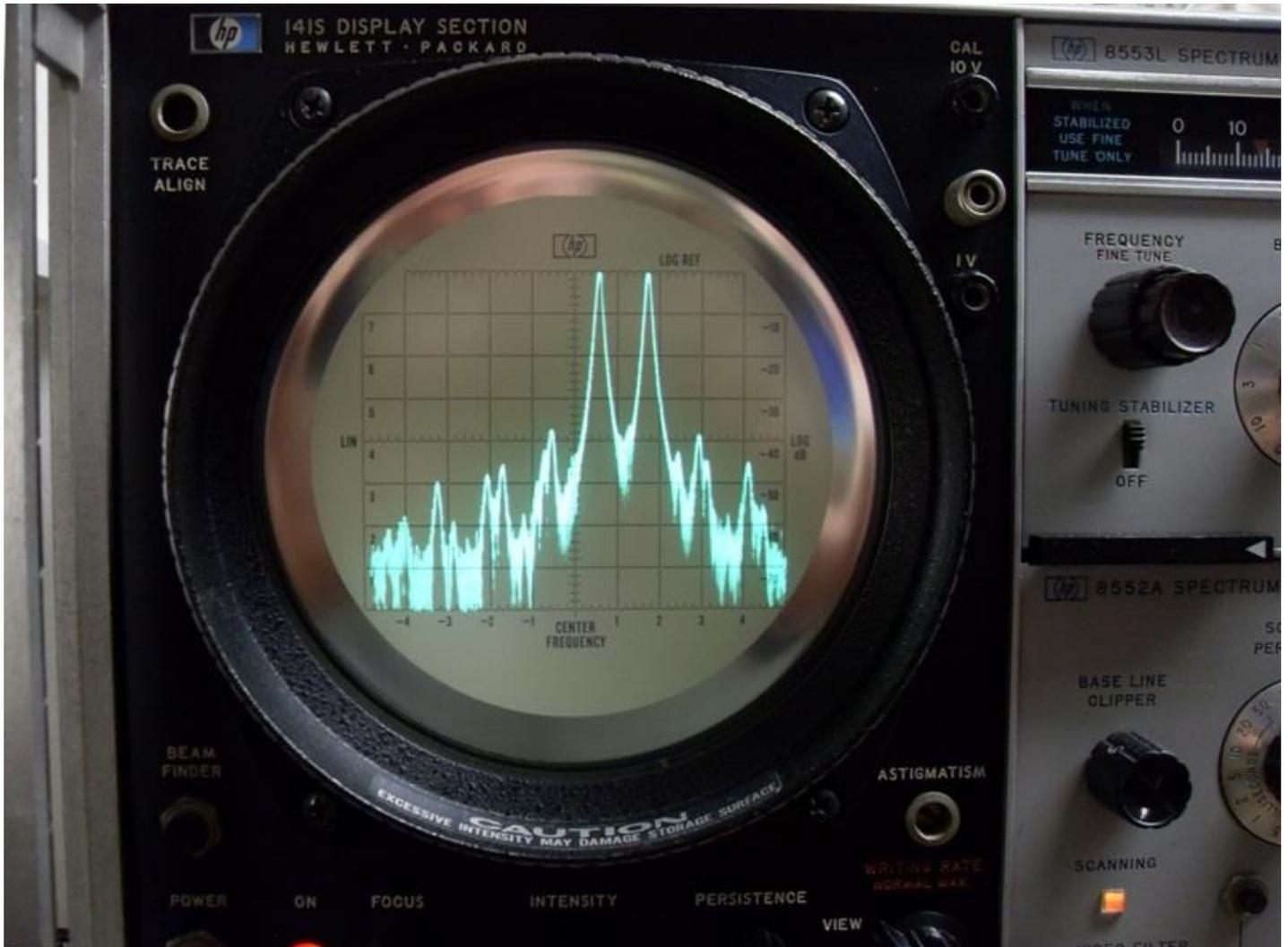
**Figure 15: Two Tone USB Output on Spectrum Analyzer. Horizontal scale is 1 KHz per division and carrier is at center. At threshold of PA grid current third order IMD products are over -30 dB and unwanted sidebands are over -45 dB.**
