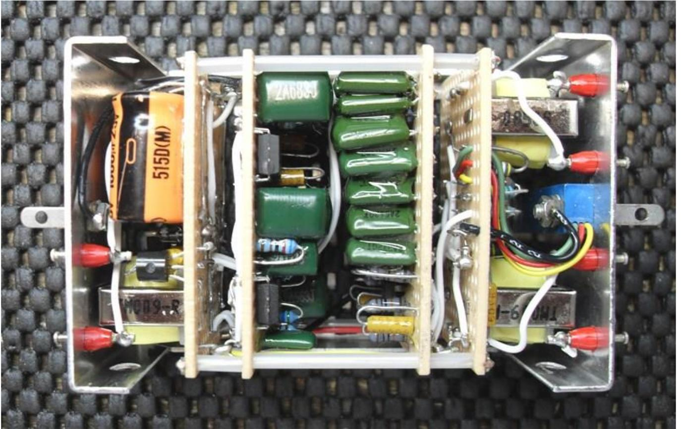
**Figure 13: The Assembled Audio Module in Minibox Enclosure**
