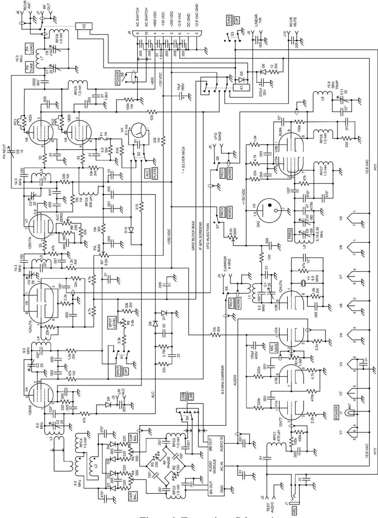
Figure 4: Transmitter Schematic
