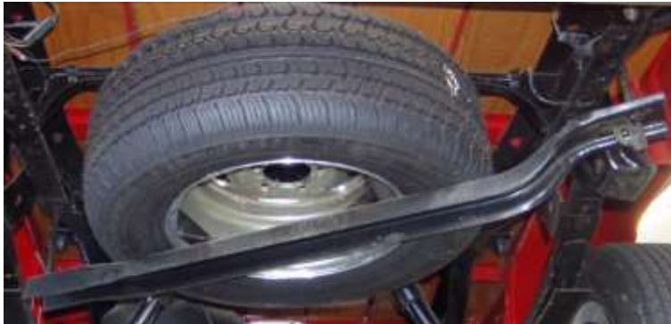
Tire carrier mounted on the truck
