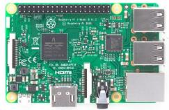
Fig.4: Raspberry Pi 3 Module
