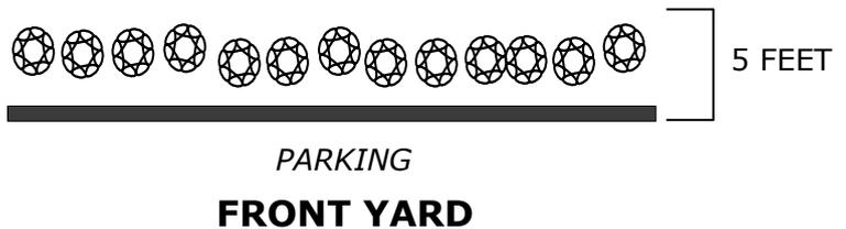
Fence, wall or berm min. 3 feet in height. Evergreen shrub, 48 inches on center, min. 30 inches in height. Class B trees, 12 feet on center, min. 6 feet in height
