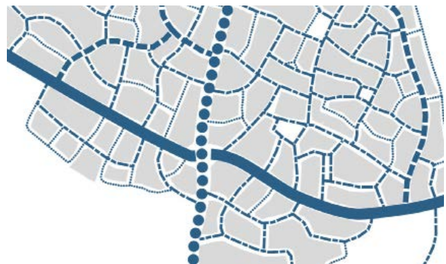
Figure 19: Example of well connected hierarchy of streets with a variety of levels linking well
