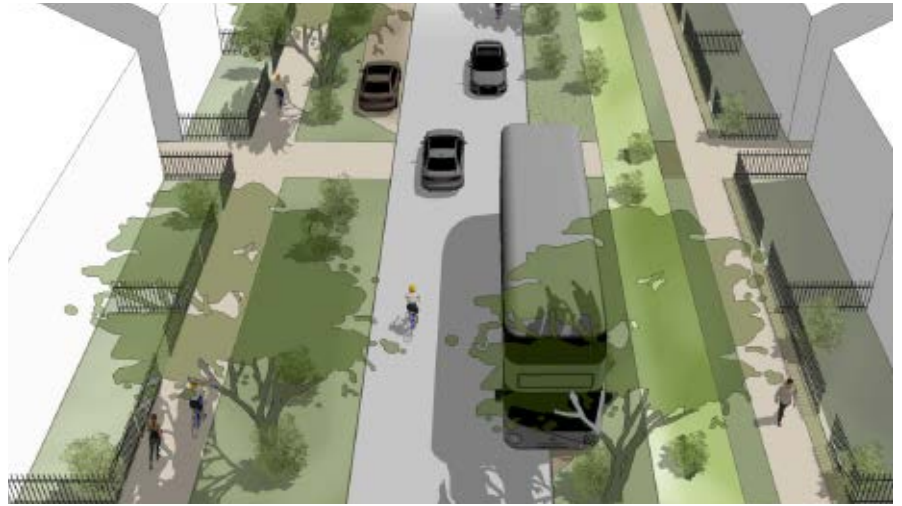
1. Min. 2m Footway 1.2 - 10m Landscaped verge Max 6 - 6.75m Carriageway excluding partially inset bus stops 1.2 - 10m Landscaped verge Foot/ Cycleway (min. 3m)
