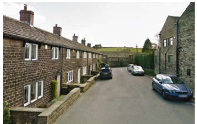
No footpaths create an informal, flexible shared street space which slows traffic speed naturally.
