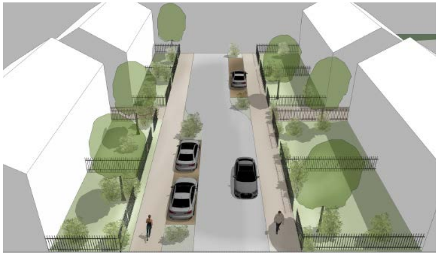
2. 2m Foot-way 1.2 - 2m Verge including parking to one side of street 4.8m Carriageway 2m Foot-way
