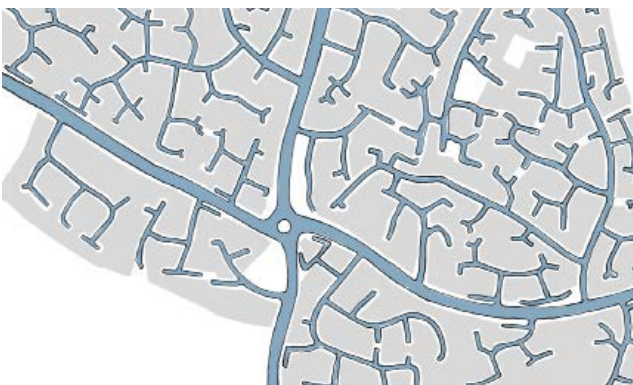
Figure 18: Example: of poorly connected street pattern with cul-de-sacs with a limited hierarchy
