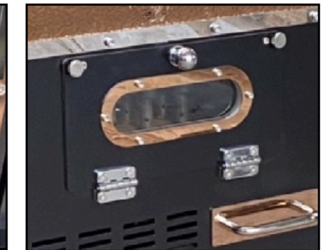
FRONT BURNER ROOM DOOR
