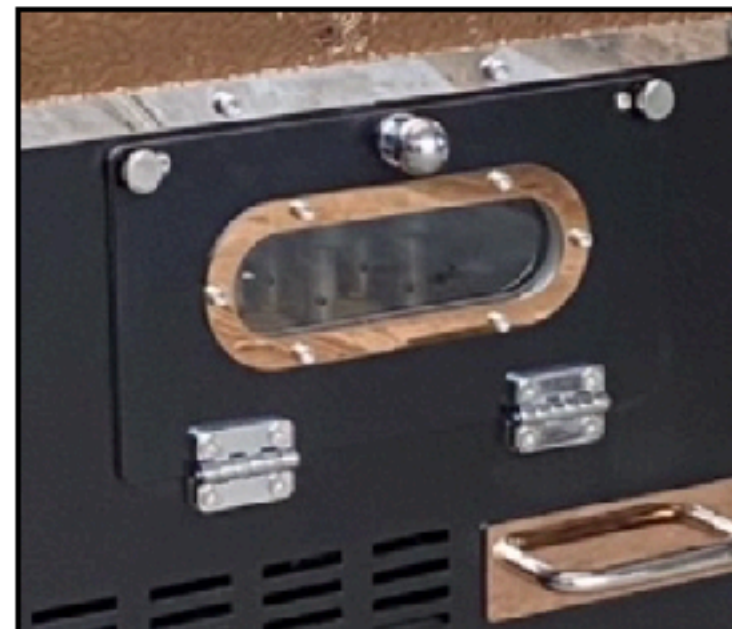
FRONT BURNER ROOM DOOR
