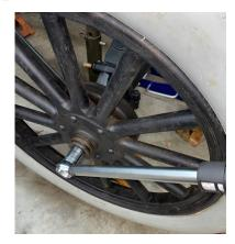
You may use a torque wrench to check the tight pull; a minimum 75 ft-lb setting is good to secure the axle nut prior to the cotter pin. After torque, pull the nut tighter to align the cotter pin hole in the axle shaft with the next slot in the axle nut. Don't pull the nut back to align the cotter pin! After 50 miles, remove the hub cap and cotter pin and check that torque setting on the axle nut for assurance that all is still tight.
