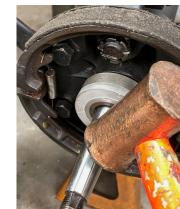
Now tap the key squarely into the keyway with a soft metal mallet. The key must be tight, without any wobble. A loose key will quickly wear the axle keyway wide, wear the hub keyway, and allow the wheel hub to become loose. A loose wheel hub may contribute to a broken axle shaft.
