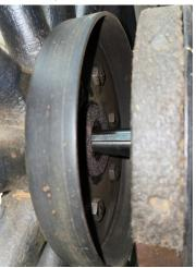
Finally, install a new axle shaft nut and tighten the nut securely. Use a new nut, as old nuts can have compromised threads. Ford used a long-handled wrench (20" length) to pull the wheel hub tight on the taper of the axle shaft with that 5/8"x18 thread axle shaft nut.
