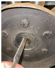
Next, select a new, unworn axle key that fits very snug to the wheel hub keyway; check to be sure the key will be a tight fit to the axle shaft keyway. Be sure to install the felt seal in the wheel hub recess to minimize axle lube leaking that may get on the brake shoes. When placing the axle key, the tapered end of the key faces the axle housing with the taper facing down into the keyway.
