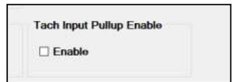
If you are connecting to an existing tachometer wire already connected to something else in the vehicle then you do not normally need to enable this. If the ECM has a software or hardware enabled pullup turned on or if a pullup is wired into the system, do not also enable this pullup (only one pullup circuit should be in use).
