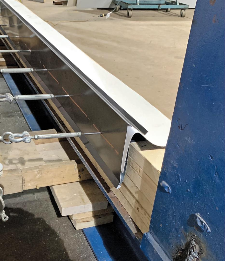
Figure 2 – RE-2 test of a fascia detail.
