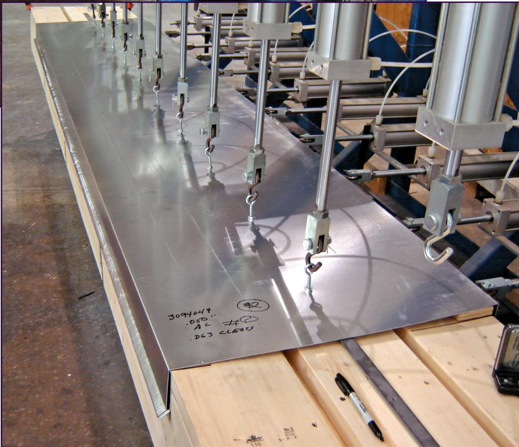
Figure 3 – RE-3 test of a coping.
