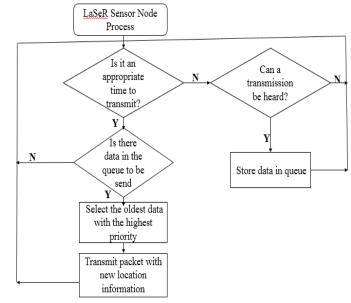
Fig.2: Flowchart of LASeR framework
