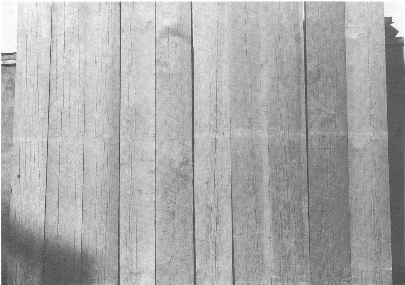
Figure 8-2—Surface checks in Douglas-fir dimensional lumber. (M 22523)
