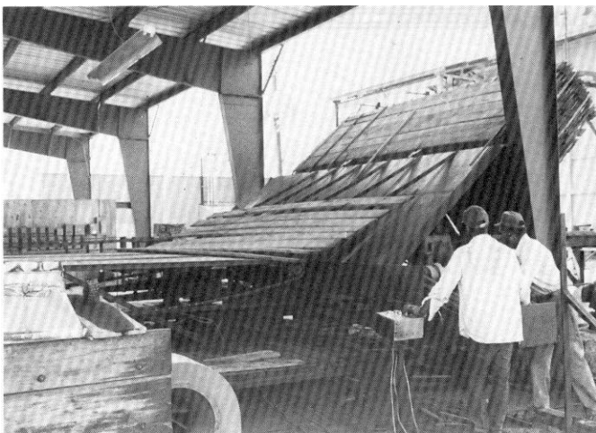
Figure 5-14—Lumber unstacker showing boards sliding onto a conveyor and stickers sliding away from the lumber. (MC88 9008)
