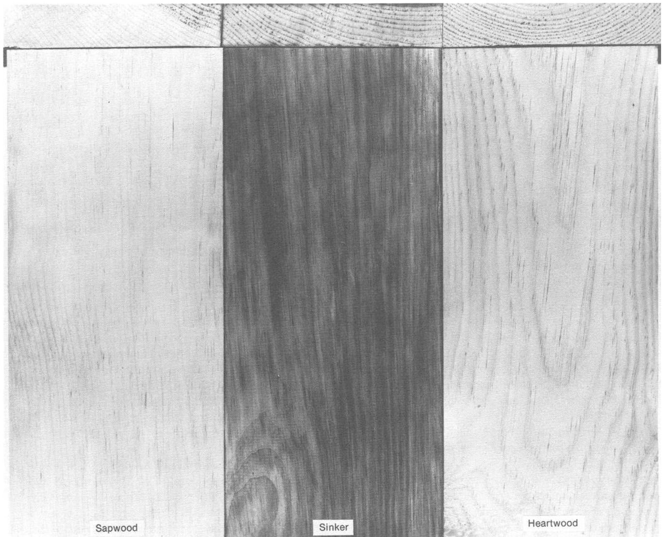
Figure 8-23—Kiln-dried sugar pine shows chemical brown stain in center board that contained wetwood but not in boards with sapwood (left) or normal heart-
