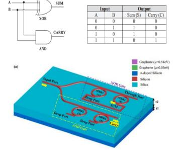
after causing interference in the two ring resonators A and B, and this part of the structure acts as an AND gate [5,6].
