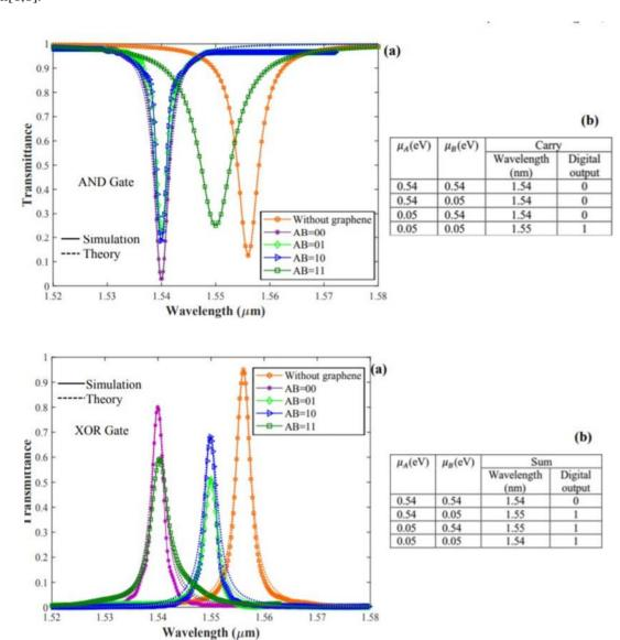
The curve of transmission versus wavelength in both numerical and theoretical simulations for the XOR gate and its Truth table.
