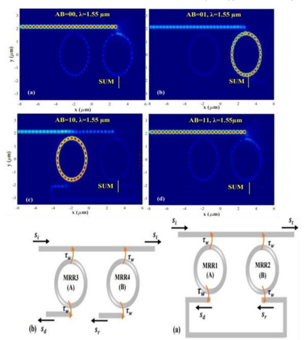
The profile of field distribution for the proposed XOR gate in different states of (a) AB = 00,
