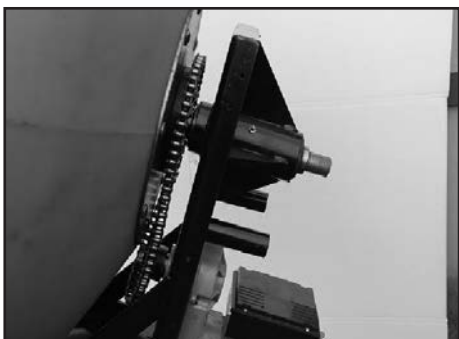
Step 6. Thread Drum into Bearing and Install Castle Nut and Install Cotter Pin.
