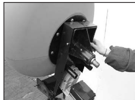
Step 8. Install Guard over Roll Chain.
