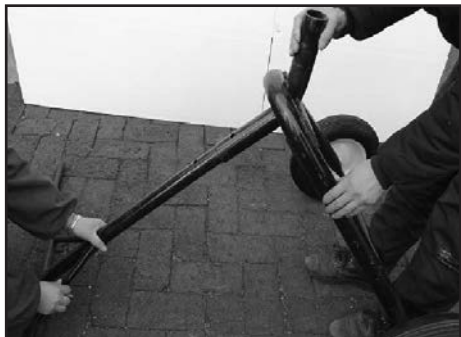
Step 3. Put Main Frame with Lower Wheel Frame and Install Bolt.
