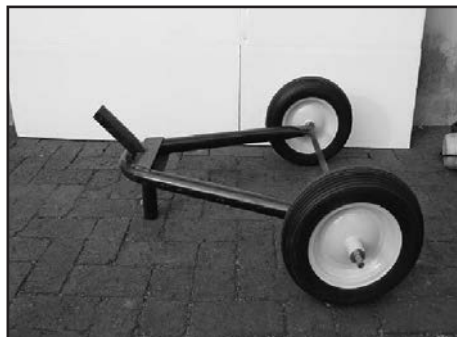
Step 1. Insert Axle in Lower Wheel and Install Wheels.
