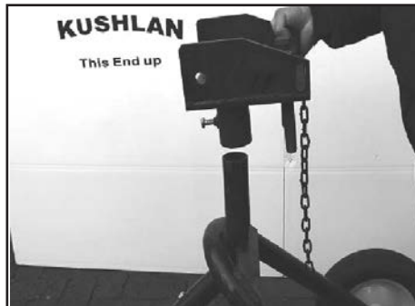
Step 4. Install Frame Pivot on Lower Wheel Frame and Tighten Bolt.
