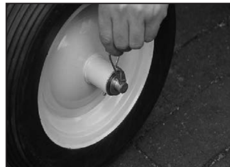
Step 2. Install R-clip in Axle.
