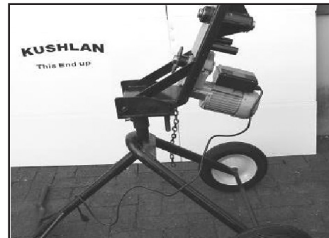
Step 5. Install Gear Box Frame with 5/8" x 10" Pivot Pin.
