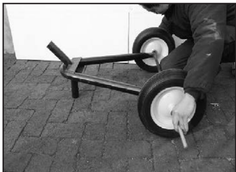
Step 1. Insert Axle in Lower Wheel and Install Wheels.
