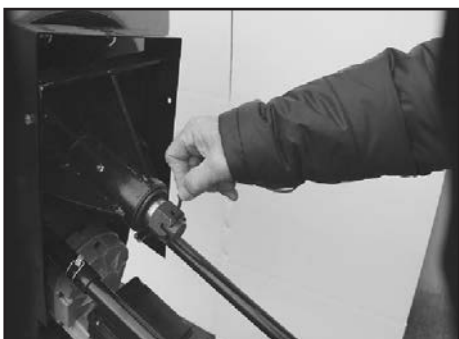
Step 9. Install Castle Nut and Cotter Pin. Note: Do Not Over Tighten Castle Nut.
