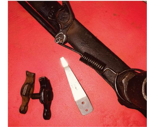
7) On the far left of this picture are two worn ratchet pawls and in the center is a new flat brake handle spring. On the far right is an accessory ratchet pawl spring - to fit one of those, open the circle end to wrap around the base of the control cross shaft, clip it shut, and place the hook end on the inside of the lever rod.
