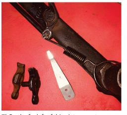
7) On the far left of this picture are two worn ratchet pawls and in the center is a new flat brake handle spring. On the far right is an accessory ratchet pawl spring - to fit one of those, open the circle end to wrap around the base of the control cross shaft, clip it shut, and place the hook end on the inside of the lever rod.
