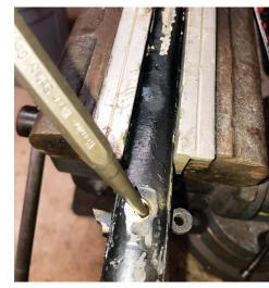
**3)** Using a punch, drive out the rivet.
