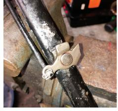
**6)** Complete the task by fitting the lever rod and inserting the cotter pin, then test the action. The brake handle's flat spring should be in good condition as well. If not, replace it or use the accessory ratchet pawl spring at the lower pawl end. Use of both is always helpful; read more in photo #7.
