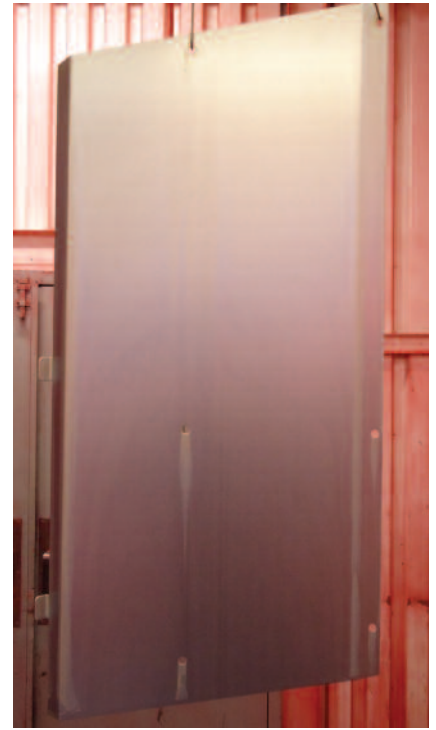
Lincoln Electric powder coats parts in a 1,500,000-square-foot manufacturing plant, operating three 8-hour shifts, 6 days a week. The part in the photo is pretreated with the new transition metal conversion.
