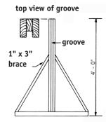
This upright consists of two pieces 1" x 3" and one piece 1" x 2", nailed together, with the 1" x 2" forming the groove for the boards to slide in.
