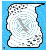
5 All discharges, whether visible or not, radiate electromagnetic signals in all directions. These signals can be monitored to determine the location and intensity of thunderstorms.
