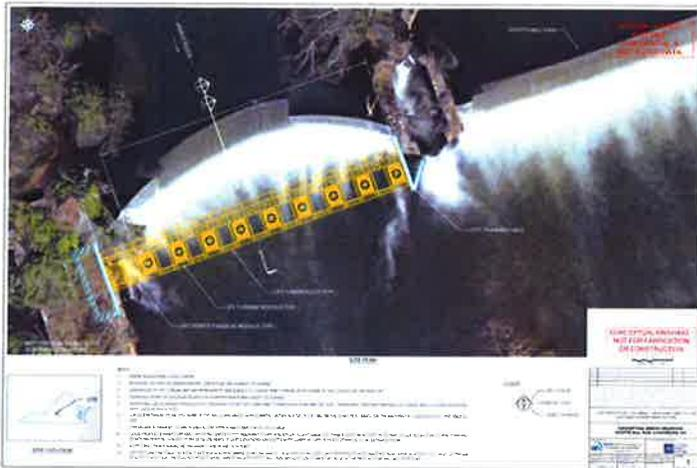
The proposed facilities would include the following: a new modular powerhouse containing nine generating units; a new 1,200-foot long underground transmission line; and three (3) appurtenant facilities, which include the addition of a 2 to 3 foot high concrete cap onto the existing spillway and raising the headpond elevation to about 517 feet.
