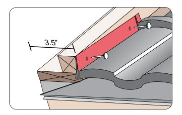
Measure, Cut & Bend-Up all rake panels against the rake build-up.
