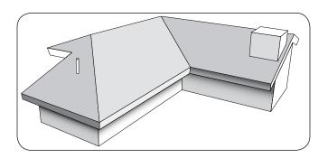
Metro Batten-less Roman panels are Installed on new or existing roofs pitched a minimum of 2-½:12 (12 degrees). An underlayment is to be installed as per local code and manufacturers instructions.
