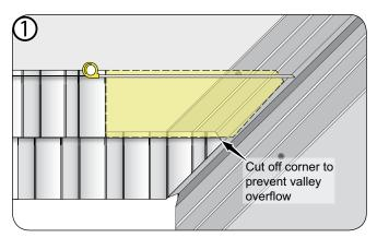
Measure, mark and cut panels to fit tightly against valley center (reverse 'V'). Fasten valley section panels to roof decking similar to the other panels without penetrating valley flashing.
