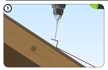
Panel back flange is fastened vertically into roof deck as shown.
