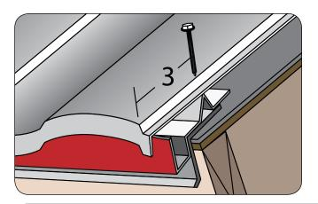
Fasten the First course up from the fascia through the top of the panel as shown. Top panel fastening is also acceptable behind Metro SMART-Vents, Chimneys and Skylights as necessary. Use fasteners with self-sealing rubber washers covered by a dome cap or seal fasteners then cover with Metro touch-up kit.
