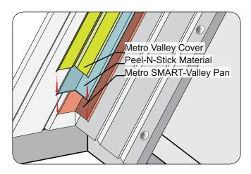
Install a strip (Min 4-in (100mm) wide) of Peel-N-Stick type material down the entire length of the valley over the center seam as shown. Install Metro Valley Cover over the center seam and stitch screw into position centered down the valley. Vertical laps for both the Peel-N-Stick and the Valley Cover are a min of 4-in (100mm).
