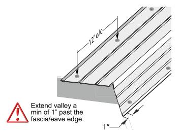
Install 20" (508mm) Double 'V' Valley metal overlapping a min. of 4" (100mm). Valleys are attached with site fabricated clips as shown. Washer and Rubber Grommet screws are acceptable at the outside locations, as shown.
