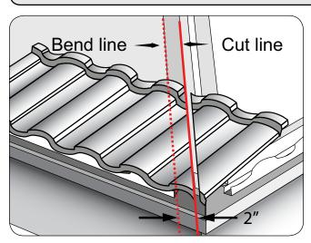
Hip cuts are measured, cut and bent in similarly to valleys. Each hip panel is bent up a min of 11/2" and fastened against the hip board.
