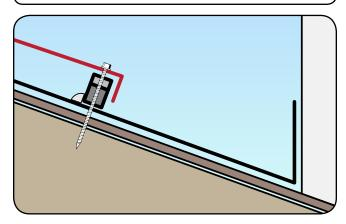
"Position the Metro XP-Foam tape and fasten as shown above.
