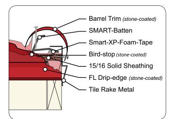
MetroTile Rake metal is installed along the rake edges as shown. This metal edging aids in positioning Metro Trim caps. Tile Rake metal is placed on the wood build-up. The Metro trim Caps cover battens and folded up Metro panel, as shown.
