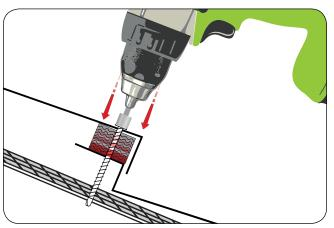
Use Metro SMART-XP-Foam tape or sealant directly beneath the area where fasteners penetrate panel.
