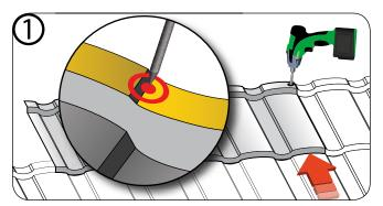
The 1st panel fastener is placed in the 'Back Flange' in the top right-hand side as shown.
