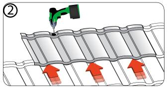
Place the 2nd panel fastener through the 'Back Flange' at the 2nd 'Under-pan' module as shown.
