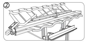
Always bend the ridge panels before cutting. Deduct 1/4" from measurements. Mark both "bend" and "cut" lines for each panel prior to cutting or bending.
