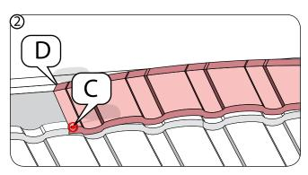
Then fasten (C) at bottom left corner and top-right corner (D) as shown. Panels are then pushed down to fit coursing properly.
