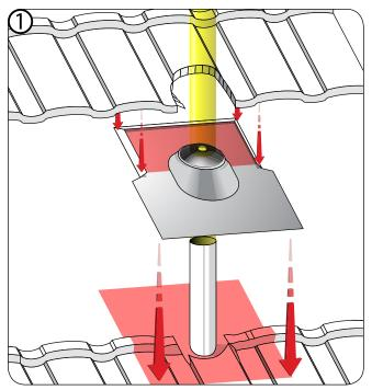
Cut panel tight to pipe and flatten the 'back-flange' portion of underlaying panel where highlighted in red above. Then seal and create a 1/2" hem around the perimeter of the SMART-Jack on the section above the pipe as shown.
