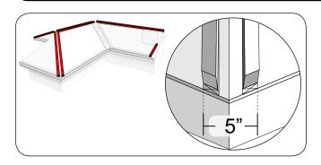
2X2 ridge battens are used to provide approximately 2" of build-up height for hip and ridge pcs. Hip battens are installed directly on top of a 1x2" spacer batten to allow cut and bent panels to be nested against the battens.
