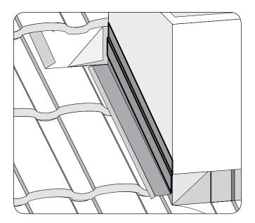
Side-wall Under-pan metal is covered with counter flashing or standard Z-bar.
