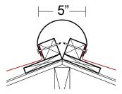
2-Trim cap fasteners in each side of cap as shown, spaced 14 ½" or on every trim cap.
