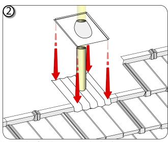
Install pipe flashing over 'Under-Pan'.
