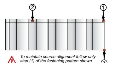
It's critical to the overall panel layout and fastening to follow the sequence shown in steps 1-3 below. Failure to do so may result in panels not being aligned or sidelaps and courses not fitting correctly.
