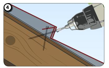
Once fastener has penetrated the nose, angle the screw to penetrate the back up-stand of the panel beneath and into the decking as shown.
