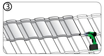
Align the overall panel and apply force as necessary to ensure the side-lap interlocks correctly, and then fasten through the 'Front Nose Downturn' on the far right-hand side of the panel as shown.
