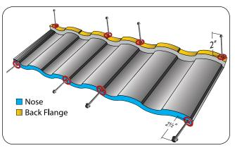
Metro Roman Batten-less panels installed direct-to-deck require front nose fasteners to be #10 x 2 1/2" long Hex Head Screws.
