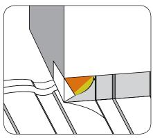
Cut and fold up panels 2" at sides of protrusion as shown.
