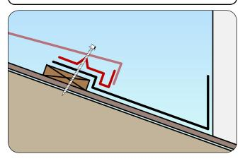
Use a V-Bat Riser Metal piece as shown to elevate the panel to the correct roof plane height. Fasten as shown with the panel nose being fastened into the V-Bat Riser.
