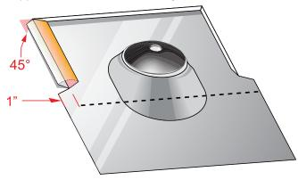
To maintain good weather protection the edges of the SMART-Jack flashing should be folded/bent up as shown to deflect any moisture onto the flashing and out onto the panel below.
