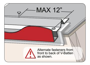
Roman panels use the "V-batten Bird-stop" which incorporates an integral 'V' batten to provide panel support at the fascia. The 'Bird-Stop' riser metal creates a 3/4" off-set from the fascia. The use of this 'Bird-stop' requires standard Drip-Edge, or Metro FL-FASCIA metal to be installed onto the roof deck first.
