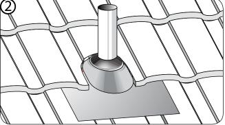
Mark, measure and cut roman panels to cover back section of SMART- jacks. Seal around flashing.
