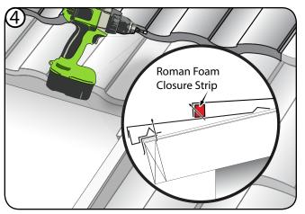
Install full panels aligned with main courses. Fasten with screws, through top panel nose through the FOAM closure strip, and into bottom panel as shown.
