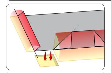
On the sides of the Chimney Saddle create side-hems to deflect water down the sides of the chimney.
