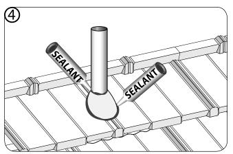
Seal Vent Pipe around bottom of cone and around pipe flashing as shown.
