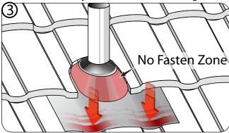
Slide the SMART-jack into place. Mold base of SMART-jack to conform with panel.
