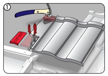
Where panels intersect with stepped fascia, stop panel battens approximately 6" from new fascia line. If necessary notch, cut, and flatten panel at this intersection as shown.
