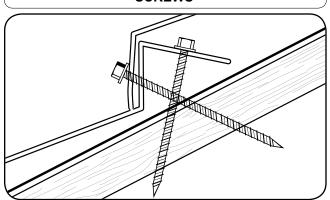
Due to the back flange and nose fastener angles, the "X" pattern provides exceptional uplift resistance.
