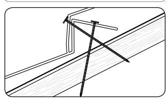
Due to the back flange and nose fastener angles, the "X" pattern provides exceptional uplift resistance.
