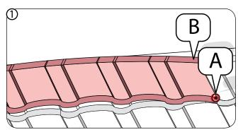
(A) Fasten first at bottom right corner, then at top-right corner (B) as shown.
