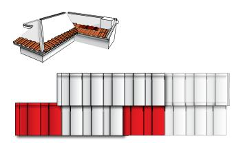
Full panels are laid from the bottom (1st full course from the fascia) up to the ridge. Batten-less Roman panels are laid from RIGHT to LEFT.
