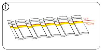
Ridge cut line is 1 " above and parallel to bend-line to allow for bend up on ridge battens.
