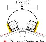
Support battens for HIP must be flush with 2X2 battens.
