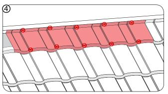
Additional fasteners are applied as necessary.
