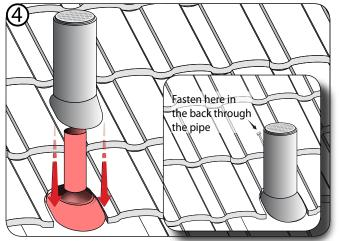
For added protection and appearance, SMART-sleeves are cut to conform to the panels and are installed over pipes. SMART-sleeves are fastened with a screw through the back of the smart sleeve into the pipe.
