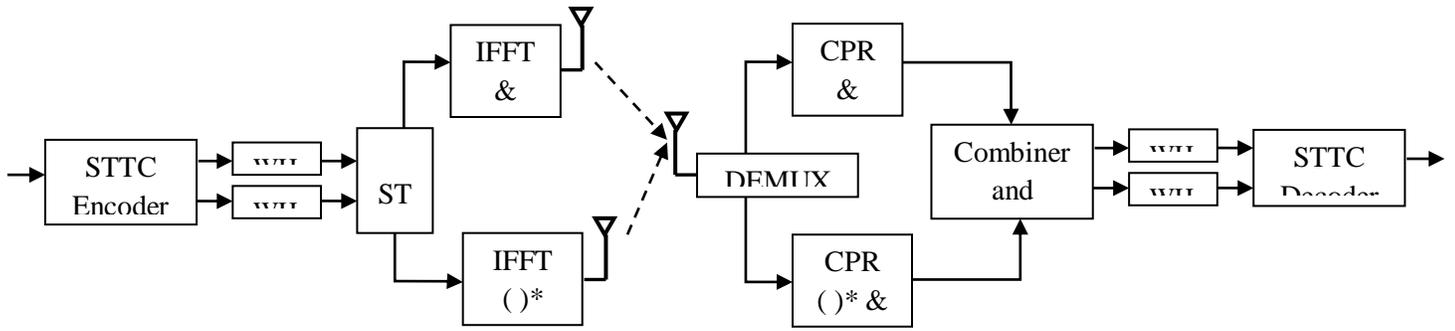
Figure 1: The architecture of a 2x1 STTC-WH-STCC-OFDM System with WHT pre-coders and CC scheme for mitigating ICI
