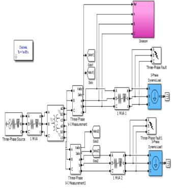
Figure 1 Simulation Model for test cases with DSTATCOM
