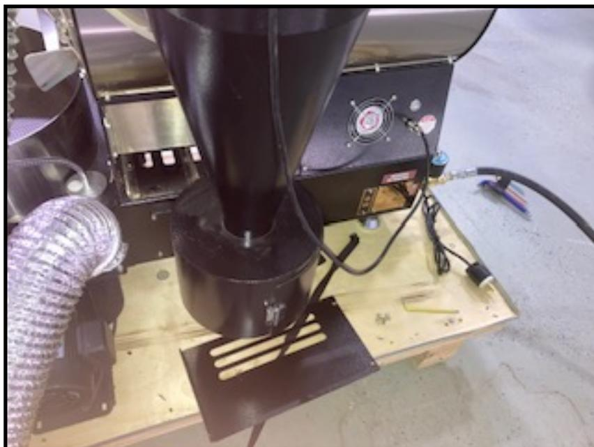
**Flexible gas line from solenoid to gas valve**
