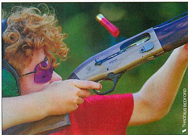
▲ A gas-operated semi-auto will tame the punch of recoil for smaller or less experienced shooters.
