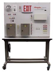
The **Model H-EM-2D** includes the following: Load Center, Control Console, Nickel-cadmium Battery, Battery Charger, Distribution Panel, Remote Control Alarm, Exit Sign Fixture, Flood Light and Wall Fixture.
