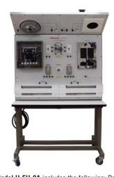
The **Model H-EH-2A** includes the following: Radiant Ceiling Lamp, Radiant Ceiling Heater, Radiant Ceiling Panel, Forced Air Wall Heater, Radiant Baseboard Heater, Low Voltage Transformer Relay, Low Voltage Thermostat and Line Voltage Thermostat.
