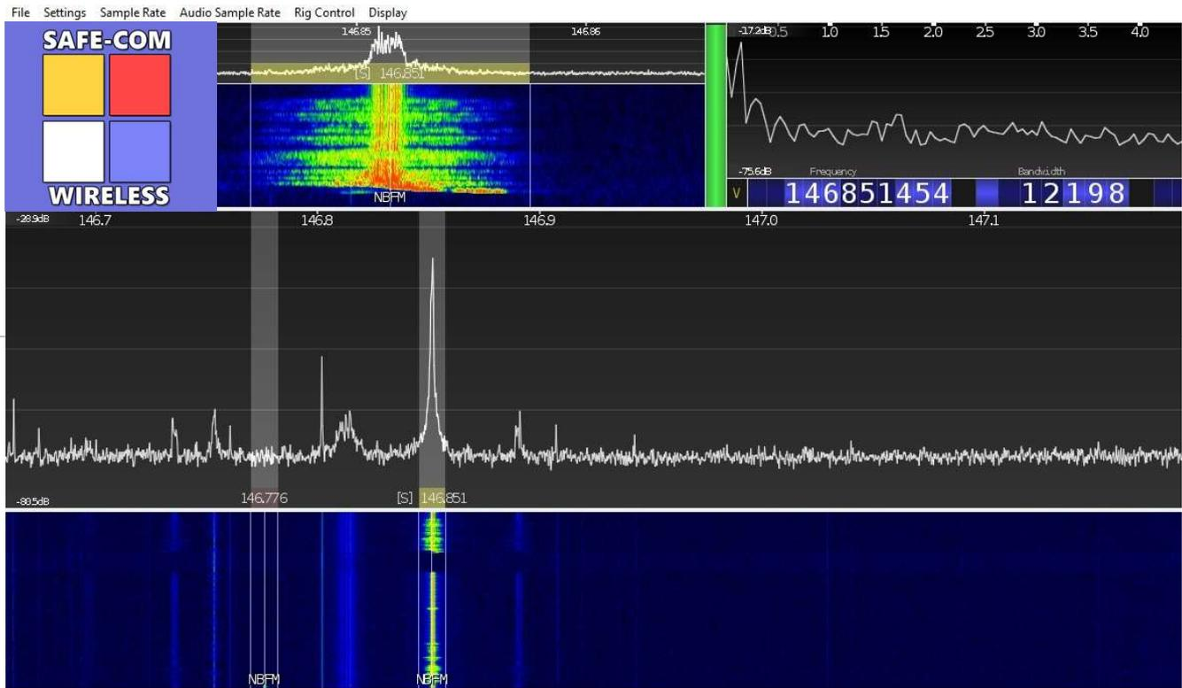
Software Define Radio based Digital Spectrum Analyzer
