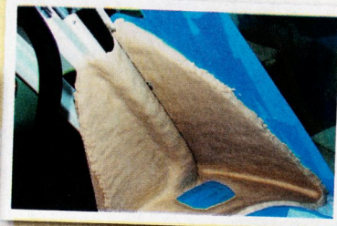
3. The initial shape of the monitor's enclosure was formed using Klean Klay (Art Chemical Products, visit www.kleanklay.com ). Notice the constant thickness of modeling clay would result in an enclosure with a gap between the dash, windshield, and all other surrounding surfaces of about 13mm (0.5 inch). Also noteworthy is the knife-edge molded into the clay at the front of the A-pillar and the clearance around the centerline of the A-pillar to allow for the routing of loudspeaker cables. The enclosure was designed to be clamped against the rubber door gasket on the back edge of the A-pillar for improved vibration isolation.
