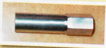
1. Two posts, containing internally threaded M5 holes on each end, were machined from aluminum. Each of these posts was anchored to a steel cross-member below the dash and supported the base monitor above the dash.
