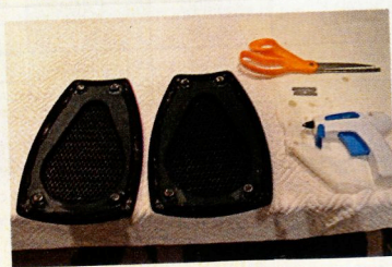
11. Speaker grilles were fabricated from 9mm (0.354 inch) marine plywood and perforated-steel sheet, which had an open area of 79 percent. The perforated steel was adhesively bonded to the marine plywood, which had generously beveled edges. Cylindrical rare earth magnets, adhesively bonded to the back of each speaker grille, allowed the grilles to be readily attached or detached from the monitors without tools. The grilles were covered with black grille cloth and a small Dynaudio logo was bonded to the lower front edge of each speaker grille. The grilles were designed mainly to protect the loudspeaker transducers from damage and should be removed for critical listening sessions.
