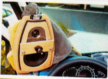
4. Once the basic shape of the enclosure was formed, the steel loudspeaker transducer mounting plate, the Sorbothane gasket, and the MDF baffle plate were mounted and carefully aimed. A magnetically attached MDF jig held a laser gun site exactly between, and on-axis with, the two loudspeaker transducers. The acoustic foam stuffed behind the baffle plate represented an attempt to reduce dipolar radiation. Literally hundreds of hours were dedicated to critical listening sessions and frequency response measurements to optimize the aim of the loudspeakers for optimal balance between soundstage width, center focus, minimization of early reflections, and tonal balance.
