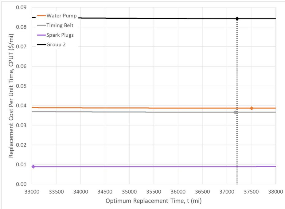
**FIGURE 4 – OPTIMUM REPLACEMENT TIMES FOR GROUP 2 AND EACH COMPONENT IN GROUP 2**
