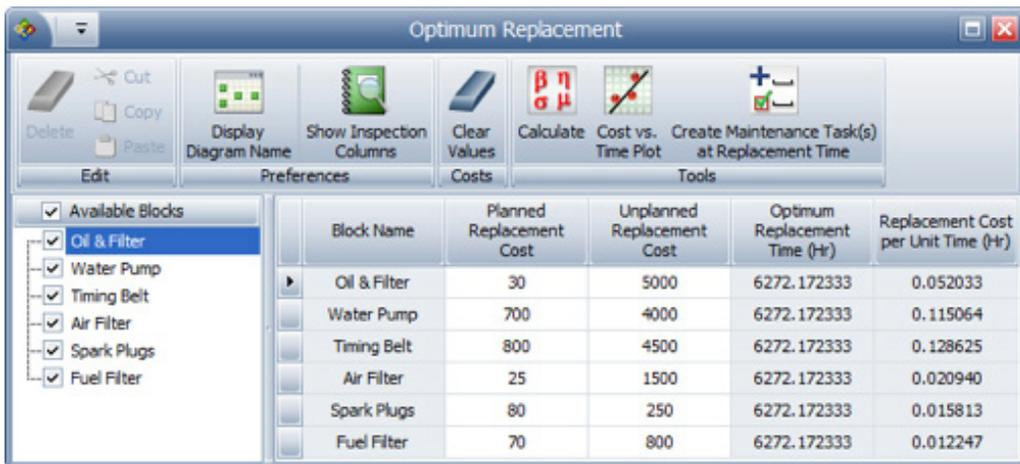
FIGURE 8 - COMMON OPTIMUM REPLACEMENT TIME AND COSTS FOR EACH COMPONENT
