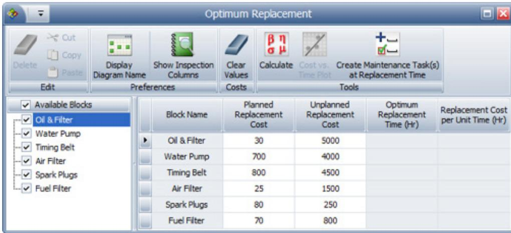
FIGURE 6 - BLOCKSIM'S OPTIMUM REPLACEMENT TOOL
