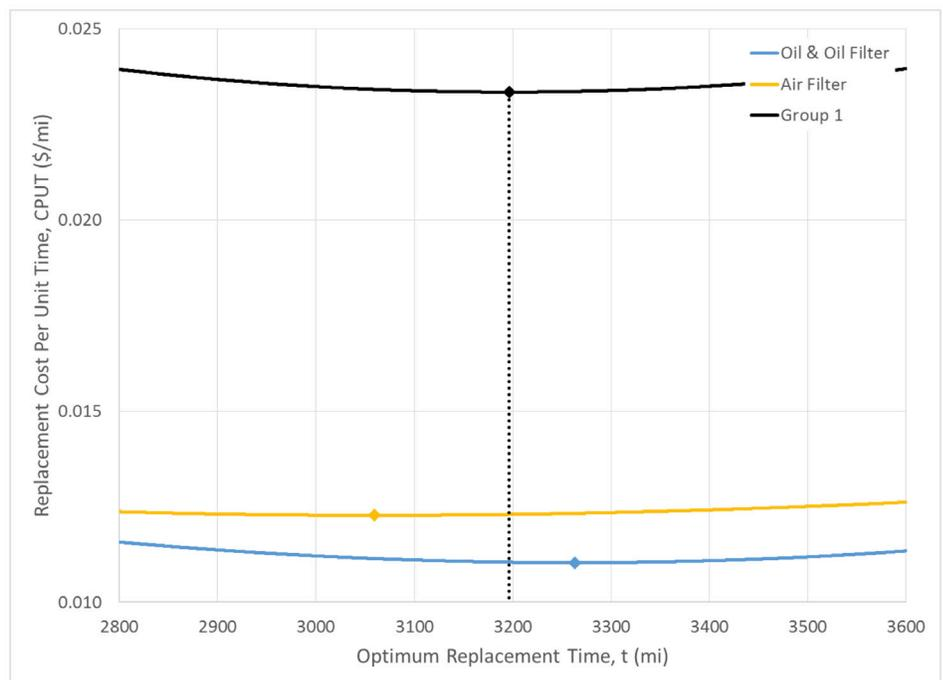
FIGURE 3 – OPTIMUM REPLACEMENT TIMES FOR GROUP 1 AND EACH COMPONENT IN GROUP 1
