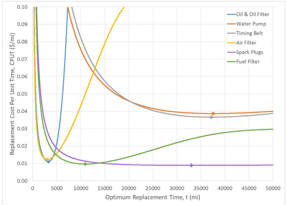
FIGURE 1 – COST PER UNIT TIME CURVES FOR EACH COMPONENT
