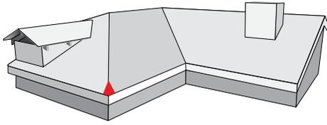
After all field panels, hip / ridge cut panels and rake cut sections are installed, the final step is to install trim caps. For Cap Cottage or Cap Shingle (2-Course) a hip starter is used at the hip / fascia corner. See steps 1-4 below and 1-3 on Page 24.
