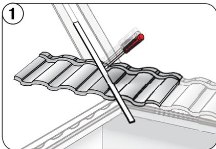
1 Measure, mark and cut panels to fit tightly against Valley center (reverse 'V').
