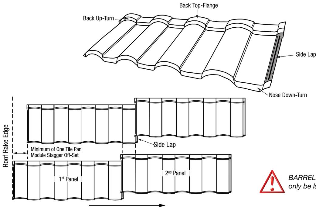
**!** BARREL-VAULT Tile panels can only be laid LEFT to RIGHT
