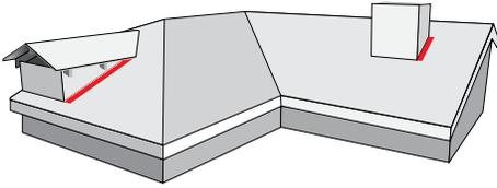
An alternative to folding panels up against sloped side walls is to use Underpan metal installed next to the wall and behind an existing wall flashing. Boral Steel Counter-Flashing metal or standard Z-Bar metal can be utilized to assist with weatherproofing where the wall flashing metal is needed.
