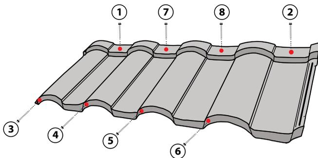
The fastening pattern for BARREL-VAULT Tile uses four (4) fasteners across the front nose down-turn and four (4) across the back up-turn of each panel.
