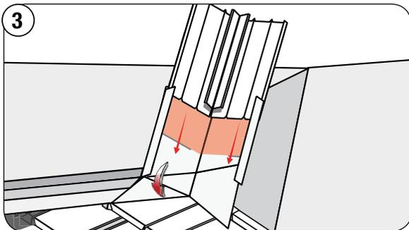
3 Install Valley metal over and onto the stone coated Flat Sheet. Apply a bead of sealant across the top of the Flat Sheet and embed the Valley into the sealant.
