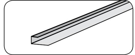
**Gutter Riser Metal / Accessory Batten**
