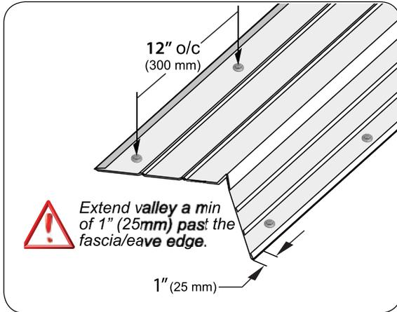
This valley metal allows for either an 'Open' or 'Closed' valley detail.
