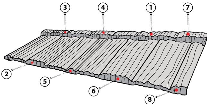
The fastening pattern for PINE-CREST Shake uses four (4) fasteners across the front Nose Down-Turn and four (4) across the Back Top-Flange of each panel.
