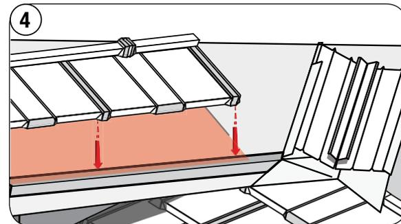
4 Then install the panels regularly as valley cut sections into the Valley 2-Pc.
