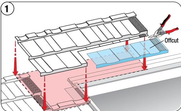
1 Cut the overhanging portion of the panel where it intersects with the stepped fascia as shown.
