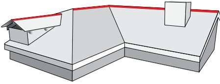
Top Row metal may be used to avoid bending and cutting full BARREL-VAULT Tile panels at the ridge.
