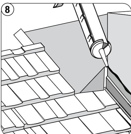
8 Install and seal Z-Bar flashing metal over folded sections as shown.
