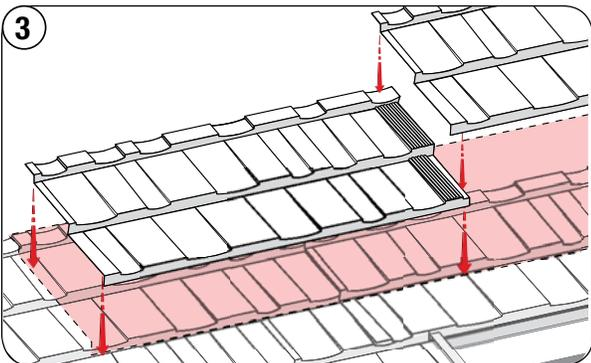
3 Apply either a bead of sealant, Barrier Foam or Foam Tape along the top surface of the under panel. Then install additional full panels half-lapping onto lower panel as shown.
