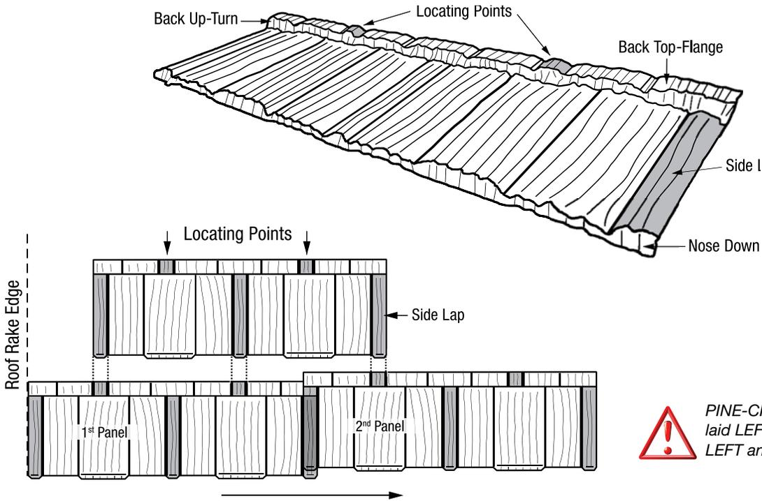
PINE-CREST Shake panels can be laid LEFT to RIGHT or RIGHT to LEFT and CANNOT be Straight-laid.
