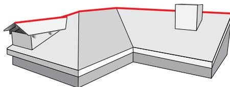
Measure, cut and install panels across ridge. Fasten as field panels. Overlapping panels is acceptable at the "horizontal" center line.
