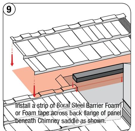
9 Install a strip of Boral Steel Barrier Foam or Foam tape across back flange of panel beneath Chimney saddle as shown.
