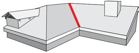
Where debris may accumulate in valleys use EmSeal Tape inserted into each piece of the two piece valley metal.
