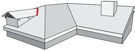
This is a critical roof area and requires special attention to ensure good weather protection. When the main roof intersects with a dormer roof, the panels back-lip where the valley exits onto the main roof must be flattened & the panels bent-up against the dormer roof (see steps below).
