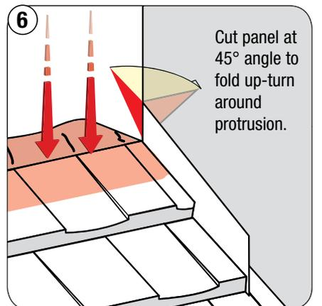
6 Flatten the back flange of the panel intersecting the top of the protrusion.
