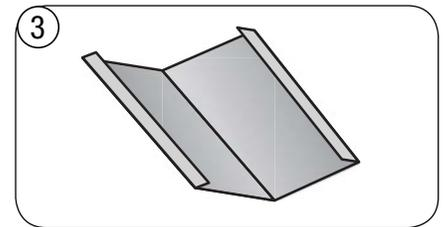
Hem both sides of the folded Flat Sheet as shown to fit around outside edges of valley.
