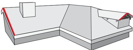
Measure, cut and install rake panel sections up each rake. Make sure to insert each section into the Rake Channel a min of .75". Refer to Panel Layout pages for correct panel lap and stagger layout.
