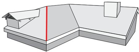
Measure, cut and fit panels to the hip center line. Overlapping panels is acceptable at the center line.
