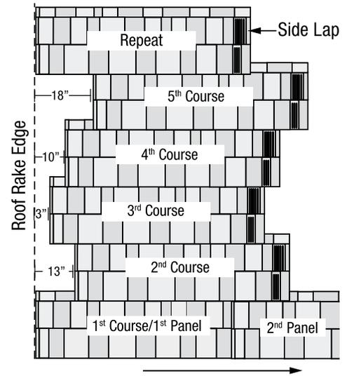
**Side Lap:** Grooved right-hand side of the panel is the "Under-Lap" portion and is covered by the "Over-Lap" of the next full panel on the same row.
