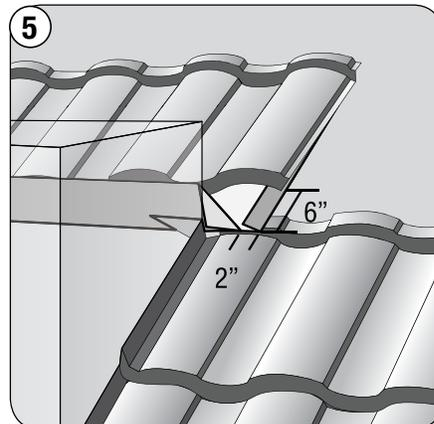
5 Apply a bead of sealant across Foam and ‘seat’ back cut-section panel onto Foam. Panels are to be fastened through front down-turn flashing, Foam and saddle into decking.
