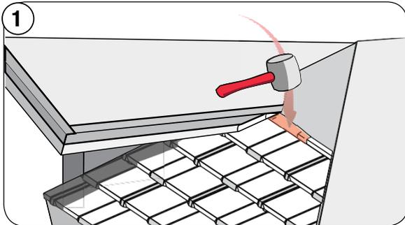
1 Flatten back flange against the roof deck.
