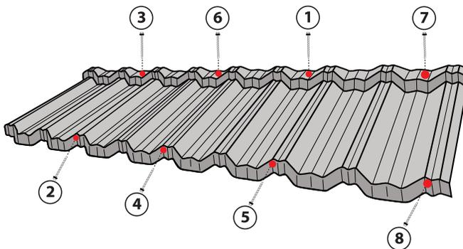
The fastening pattern for PACIFIC Tile uses four (4) fasteners across the front Nose Down-Turn and four (4) across the Back Top-Flange of each panel.
