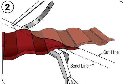
2 Mark the bend line 1 1/2" in from the cut line (1" bend down when installed batten-less).
