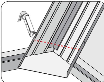
Apply a bead of sealant atop the Flat Sheet and seat the Valley Metal as shown.
