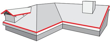
Install the BARREL-VAULT Tile Bird-Stop Riser across the fascia on top of a 1x4 Support Batten. The positioning is critical as this part will dictate panel layout across the roof, as the panels follow the scalloped profile of the Bird-Stop.
