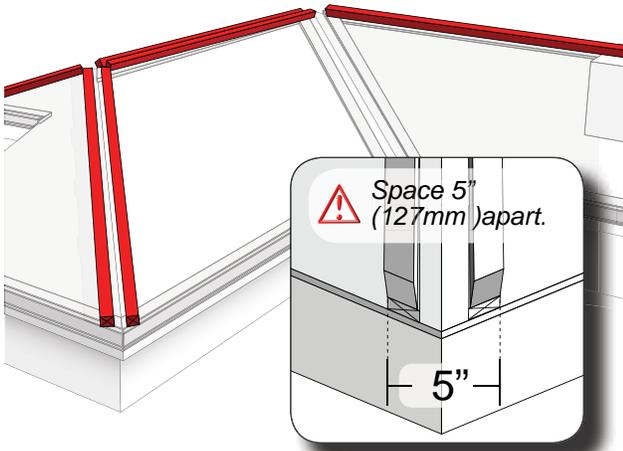
Ridge & Hip battens can be positioned side by side, or vertically stacked as shown, using either 2x2, 1x4 or combination of both. They are used to provide approximately 1.5 inch of build-up height from hip and ridge pieces. Hip battens are installed directly on top of intersecting panel battens if used, so the panel cut sections can be fitted against the battens.
