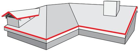
Boral Steel Batten-less panels are installed on new or existing roofs pitched a minimum of 3:12 (12 degrees). Underlayment is to be installed as per local code and manufacturer's instructions.
