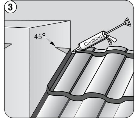
3 At back of chimney, seal each top corner section. Keep panel battens away from saddle as shown.
