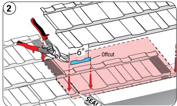
2 Lap the first cut-panel with a new full panel and cut/remove the section and seal as shown.
