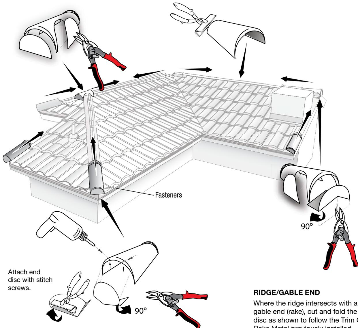
Attach end disc with stitch screws.
