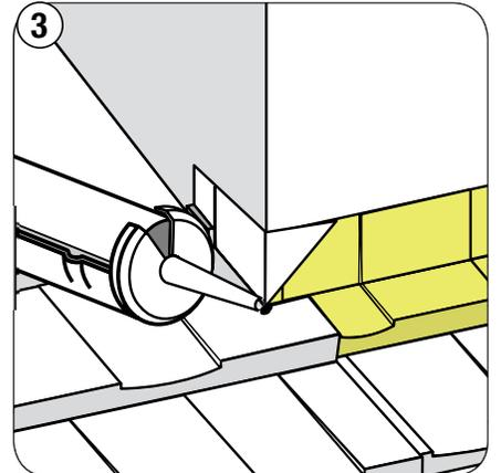
3 Cut and fold up panels 2" at sides of protrusion. Seal corner laps as shown.
