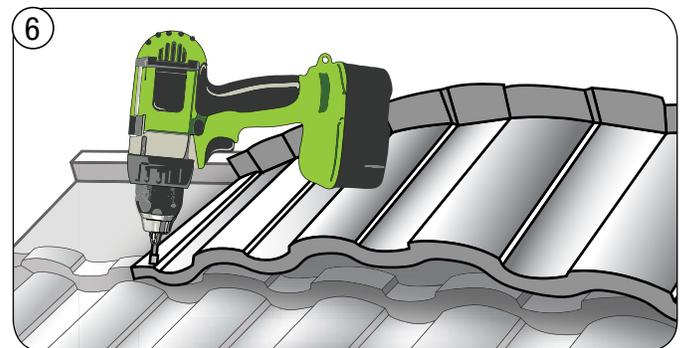
Then fasten at bottom far left corner. Panels are then pushed down to fit coursing properly.
