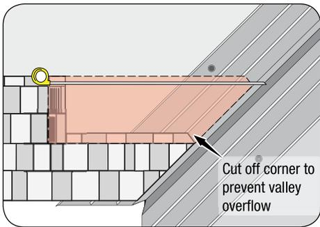
Measure, mark & cut panels to fit tightly against Valley center (reverse 'V'). Fasten valley section panels to roof decking similar to the other panels without penetrating valley flashing.
