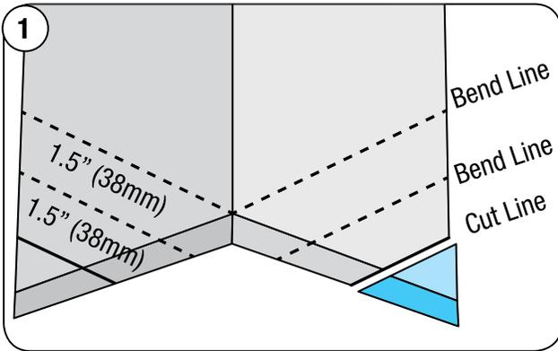
1 Mark cap as shown at center point. mark lines with 1.5" (38 mm) of spacing.
