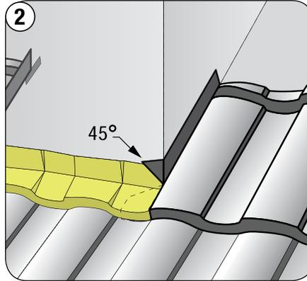
2 Cut 45° angle and fold tabs around chimney.
