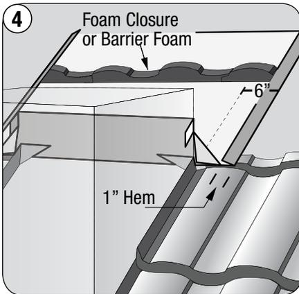
4 At back of chimney, install chimney saddle as shown. Extend saddle a minimum of 4” (100 mm) past each side of chimney. Hem ends 1” (25 mm) to keep water on saddle flashing.
