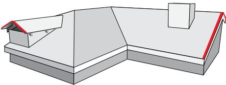
Boral Steel Trim Cap Rake Metal is installed along the rake edges as shown. This metal edging aids in positioning Boral Steel Trim Caps.
