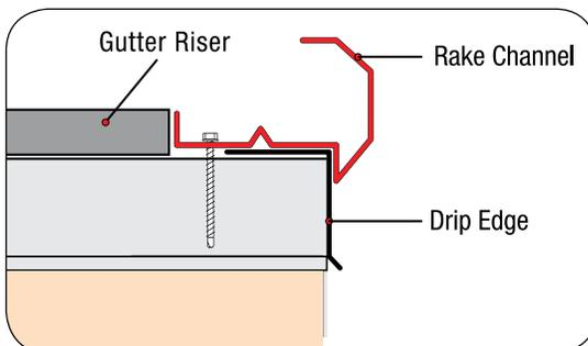
Install the Boral Steel Rake Channel using fasteners placed as shown. If fasteners do not have a sealing washer, apply a bead of sealant around each one. Rake Channel metal is notched to lap a minimum of 2" (50 mm) with water flow, as shown.
