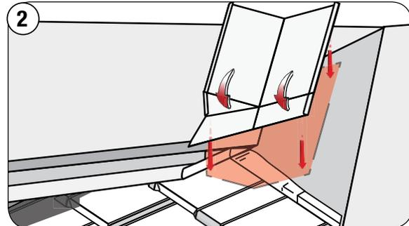
2 Form the stone coated Flat Sheet as an extension and exit tray for the upcoming valley. Apply sealant under the Flat Sheet where it exits on top of the panel beneath.
