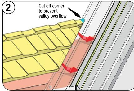
2 Notch the top Back Flange corner prior to fitting into the Valley.
