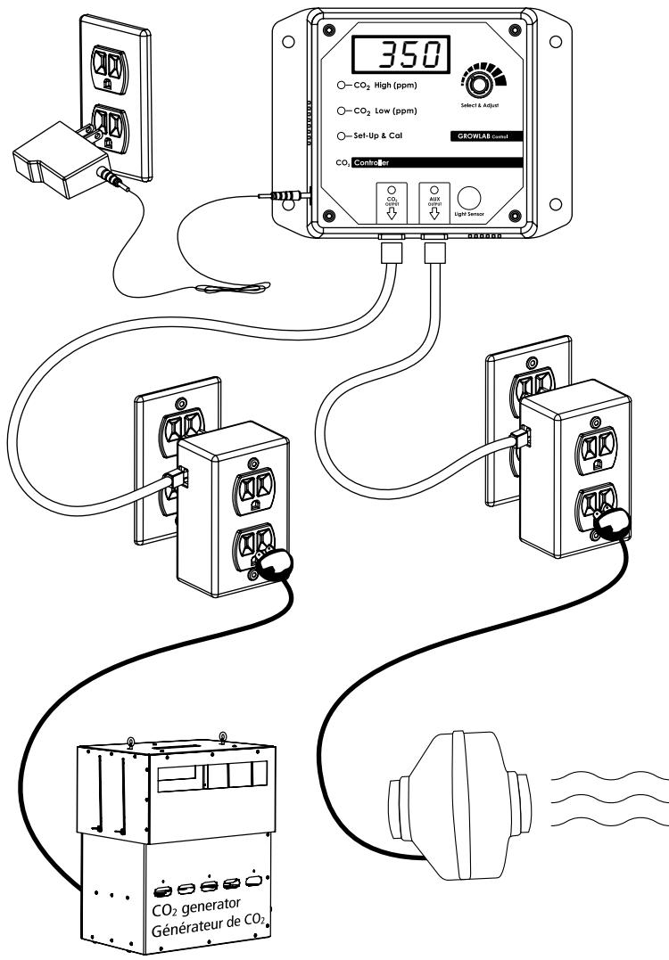
Place Controller on a wall at plant level.
