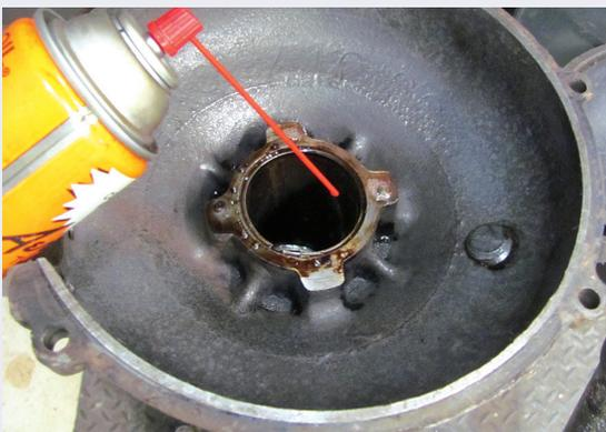
Clean the 'V' slit in the sleeve and look at it carefully. When using the puller, that slit needs to collapse to remove the sleeve. Turn in the direction of the red arrow in the picture below, twisting the sleeve while pulling. The narrow 'V' will then twist into the larger 'V' to shrink the sleeve for removal.
