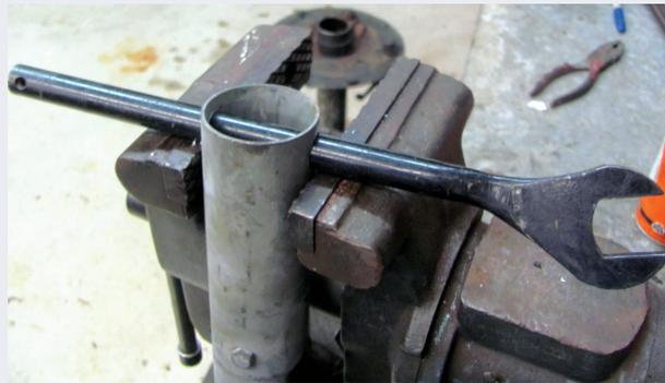
Take care to clean out old grease and use lots of penetrating oil, too. Clean the grease cup hole, as the puller tool spring 'button' needs to engage in that hole.
