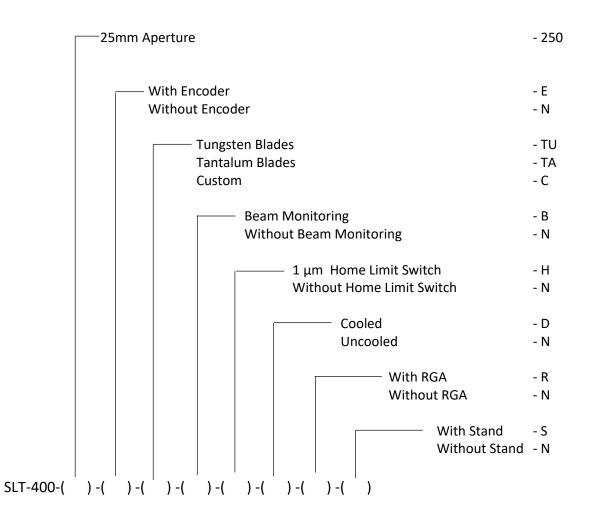
For example, a chamber configured with 25mm Apperture, with an Encoder, Tungsten Blades, without beam monitoring, 1  $\mu$ m Home Limit Switch, Cooled, without RGA and a Stand would be denoted by: SLT-400-250-E-T-N-H-D-N-S
