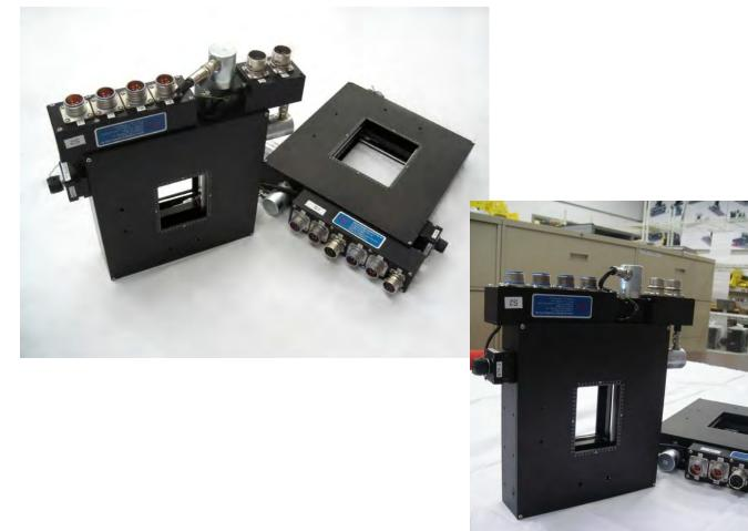
ADC custom designed and built two slits for PELICAN instrument located at ANSTO Neutron facility. The blades are mounted on preloaded carriages that are guided by miniature ball guide rails. The blades are fully scannable. A Kubler Absolute Multiturn Rotary Encoder is used to track the position of the blades. The limits are lever style snap-action switches. Connectors are circular MIL Spec Metal Connectors as specified by the customer.
