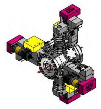
Blades are actuated independently by 4 actuators mounted on the slit body. This slit system was designed to be robust and easily serviceable.
