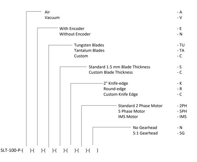
For example, a chamber configured for Air, No Encoder, Tungsten Blades, Standard Thickness, No Beam Monitoring, Standard 2 Phase Motor, with no gearhead would be denoted by: SLT-100-P-A-N-TU-S-K-2PH-N.
