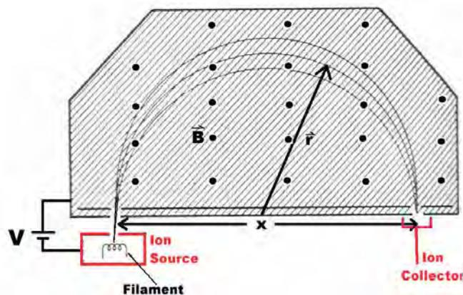
Figure 9 - Principles of a helium leak detector sensor.
