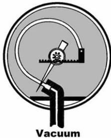
**Figure 3 - Mechanical Gauge (Bourdon type)**
