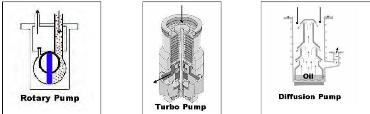
Figure 7 – Three types of vacuum pumps; rotary (mechanical), turbomolecular (mechanical) & oil diffusion
