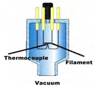
**Figure 4 - Thermocouple Gauge**
