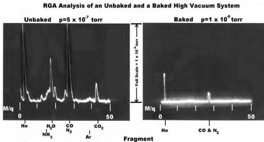
Figure 11 - RGA Spectra for an unbaked and baked HV system.
