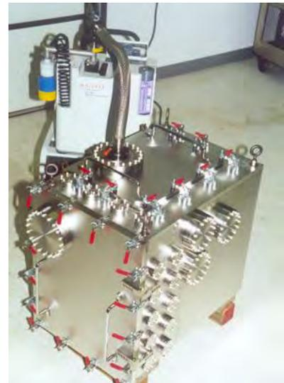
**Figure 1 - An ultra-high vacuum chamber being evacuated with a turbomolecular pump.**
