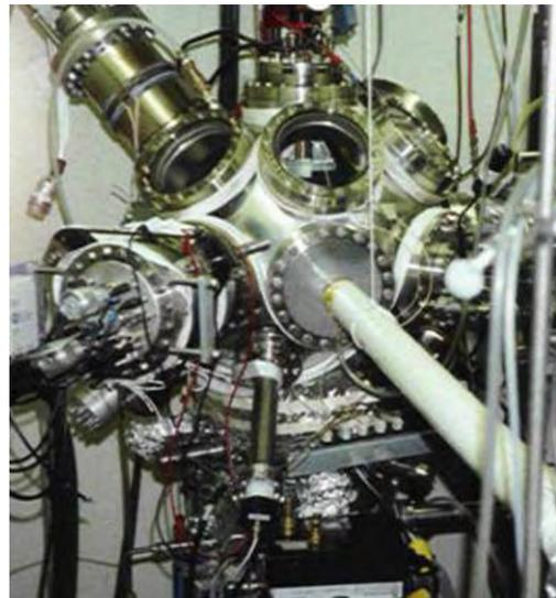
**Figure 12 - The author's double-walled XHV chamber with white bake-out heater tapes exposed. Internal IR heating lamps do the bulk of the work of removing internal adsorbates.**
